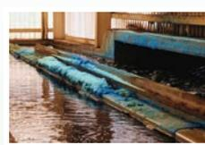
Bioleaching of copper from copper sulfide ores at the Skouriotissa copper mine in Cyprus.
