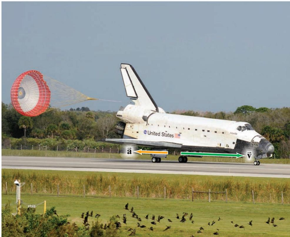
The space shuttle has released a parachute to reduce its speed quickly. The directions of the shuttle's velocity and acceleration are shown by the green ( $\vec{v}$ ) and gold ( $\vec{a}$ ) arrows.
