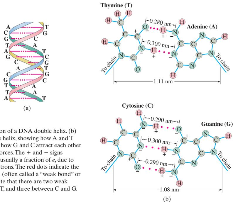
**FIGURE 47** (a) Section of a DNA double helix. (b) “Close-up” view of the helix, showing how A and T attract each other and how G and C attract each other through electrostatic forces. The + and – signs represent net charges, usually a fraction of  $e$ , due to uneven sharing of electrons. The red dots indicate the electrostatic attraction (often called a “weak bond” or “hydrogen bond”). Note that there are two weak bonds between A and T, and three between C and G.
