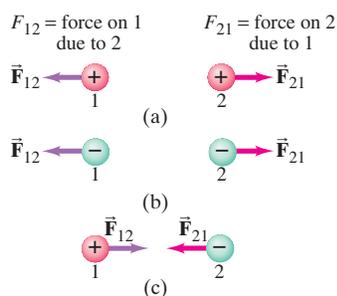
**FIGURE 15** The direction of the static electric force one point charge exerts on another is always along the line joining the two charges, and depends on whether the charges have the same sign as in (a) and (b), or opposite signs (c).
