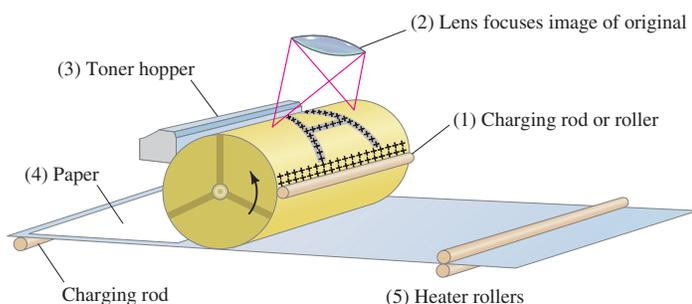
**FIGURE 49** Inside a photocopier machine: (1) the selenium drum is given a + charge; (2) the lens focuses image on drum—only dark spots stay charged; (3) toner particles (negatively charged) are attracted to positive areas on drum; (4) the image is transferred to paper; (5) heat binds the image to the paper.
