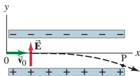
**EXAMPLE 16 Electron moving perpendicular to  $\vec{E}$ .** Suppose an electron traveling with speed  $v_0$  enters a uniform electric field  $\vec{E}$ , which is at right angles to  $\vec{v}_0$  as shown in Fig. 41. Describe its motion by giving the equation of its path while in the electric field. Ignore gravity.
