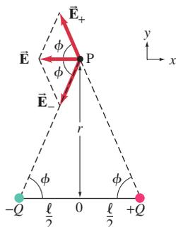
**FIGURE 45** Electric field due to an electric dipole.
