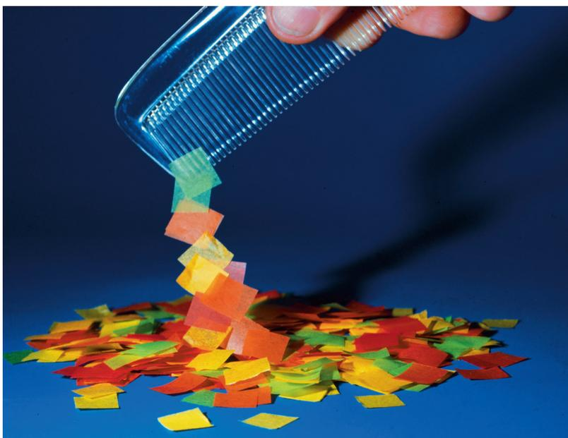
This comb has acquired a static electric charge, either from passing through hair, or being rubbed by a cloth or paper towel. The electrical charge on the comb induces a polarization (separation of charge) in scraps of paper, and thus attracts them.
