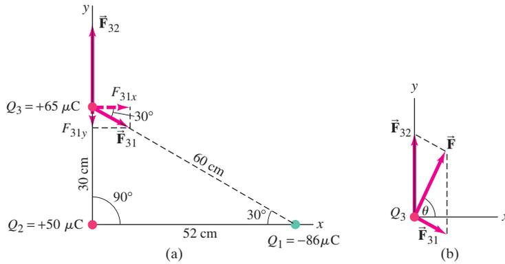
**FIGURE 18** Determining the forces for Example 3. (a) The directions of the individual forces are as shown because  $\vec{F}_{32}$  is repulsive (the force on  $Q_3$  is in the direction away from  $Q_2$  because  $Q_3$  and  $Q_2$  are both positive) whereas  $\vec{F}_{31}$  is attractive ( $Q_3$  and  $Q_1$  have opposite signs), so  $\vec{F}_{31}$  points toward  $Q_1$ . (b) Adding  $\vec{F}_{32}$  to  $\vec{F}_{31}$  to obtain the net force  $\vec{F}$ .
