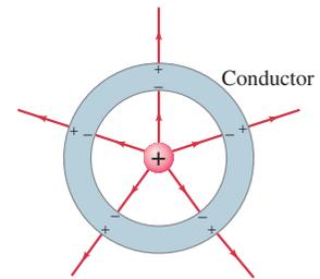
FIGURE 36 A charge inside a neutral spherical metal shell induces charge on its surfaces. The electric field exists even beyond the shell, but not within the conductor itself.
