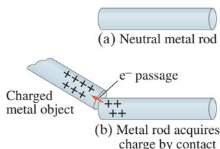
**FIGURE 6** A neutral metal rod in (a) will acquire a positive charge if placed in contact (b) with a positively charged metal object. (Electrons move as shown by the orange arrow.) This is called charging by conduction.
