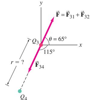
**FIGURE 19** Example 4:  $Q_4$  exerts force ( $\vec{F}_{34}$ ) that makes the net force on  $Q_3$  zero.
