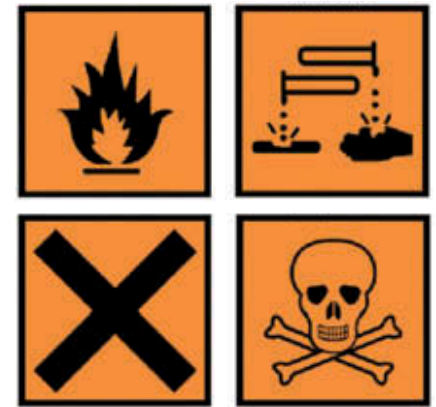
Figure 2.7 Hazardous substance symbols showing that materials are flammable, corrosive, harmful/irritant or (very) toxic
