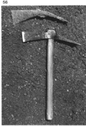
56 An ancient kivel or stone-mason's hammer and a modern one at Pompeii. The continuity in the form of this tool is remarkable.
