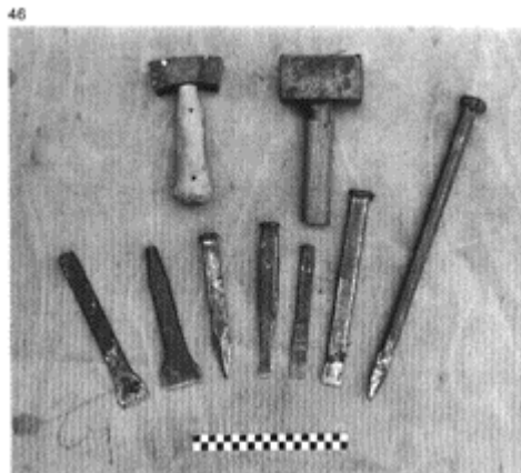
46 The principal tools of the stone-mason remained the same from the Roman period up to the twentieth
