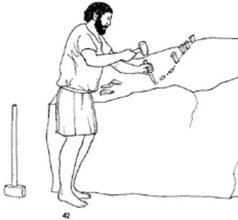
42 Drawing showing splitting a block using wedges.
