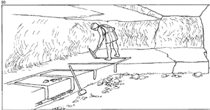
30 Reconstruction of quarrying in galleries in the tufa of Grotta Oscura (Latium).
