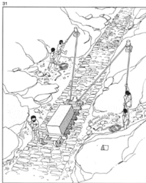
31 The descent of marble blocks from the quarry on Pentelikon. (After A.K.Orlandos.)
