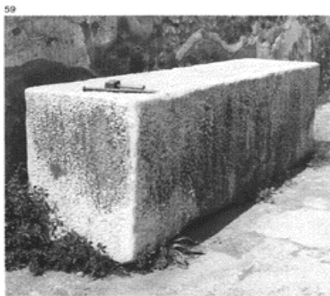
59 A roughed-out block of white limestone, brought from the quarry with scabbled facings, intended for the reconstruction of the Forum at Pompeii after 62. Length: 3.07m; width: 0.73m; height: 1m; weight 5800kg.
