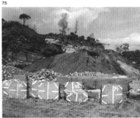
75 Marks painted by the quarrymen to distinguish the destination of the stones. Lava quarry of Terzigno. The practice of marking stones to indicate their destination was already standard in ancient quarries.
