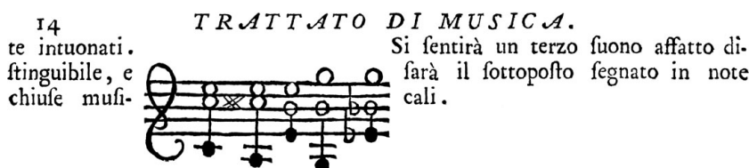
Figure 1.4 Tartini’s 1754 publication of his observation of un terzo suono , a third sound, shown as filled notes below the first two sounds playing on violins or horns—among the earliest recognitions of a nonlinear effect in hearing. The note pitches that Tartini illustrated represent the ratios 4:5:2, 5:6:2, 3:4:2, 5:8:2, and 3:5:2 ( f_1 : f_2 : f_3 , for f_1 being the pitch of the lower played sound and f_2 being the pitch of the upper one, and f_3 being the pitch of the low third tone). The third-tone pitch corresponds to the quadratic intermodulation product f_2 - f_1 , or the cubic intermodulation product 2f_1 - f_2 , and/or an octave above one of those. As Helmholtz (1863) remarked of these observations, “It is very easy to make a mistake of an octave. This has happened to the most celebrated musicians and acousticians. Thus it is well known that Tartini, who was celebrated as a violinist and theoretical musician, estimated all combinational tones an octave too high.” Sorge’s 1745 observation of c'' and a'' making an f would be 3:5:1, with den dritten Klang , a third-order (cubic) distortion product, at 2f_1 - f_2 .
