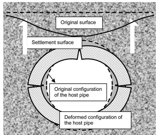
Figure 11. Stress distribution accompanying deterioration of the host pipe.
