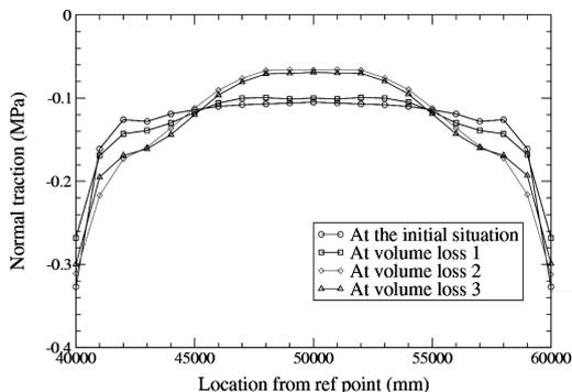
Figure 5. Normal traction on rough foundation for different values of volume loss (Boonpichetvong, Netzel & Rots).
