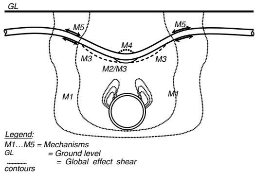
Figure 5. Schematic representation of five global and local mechanisms (Vorster et al.).
