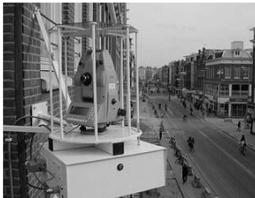
Figure 17. Automated total station in use for monitoring North-South line tunnel construction project in Amsterdam (Van der Poel et al, 2005).
