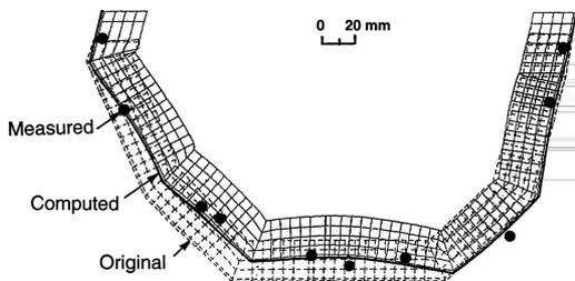
Figure 19. Computed and measured deflections.
