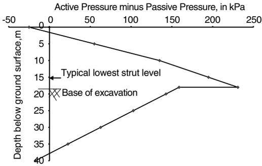
Figure 5. The ‘net active’ pressure on the wall of an 18 m deep excavation. The undrained strength profile used is that for Clarke Quay in Figure 3.
