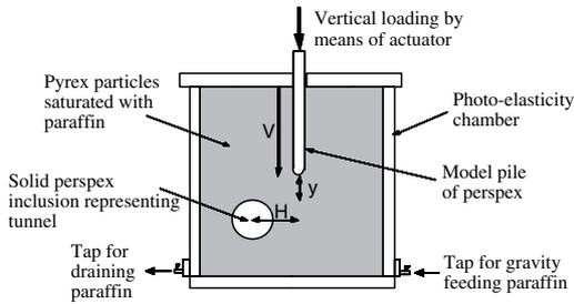
Figure 1. Test set-up (Standing & Leung, 2005).
