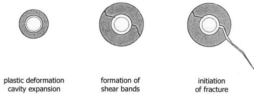
Figure 15. Hydraulic fracture initiation in sand.
