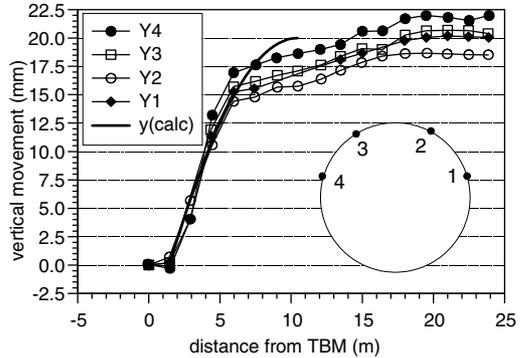
Figure 7. Vertical movement of tunnel lining segment immediately after erection (Bezuijen and Talmon, 2005).
