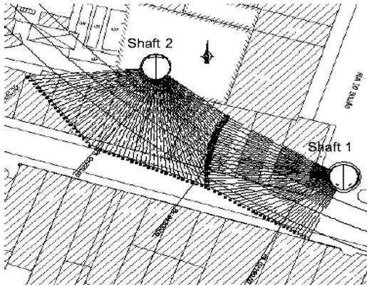
Figure 12. Plan of the sub-horizontal grout injection.
