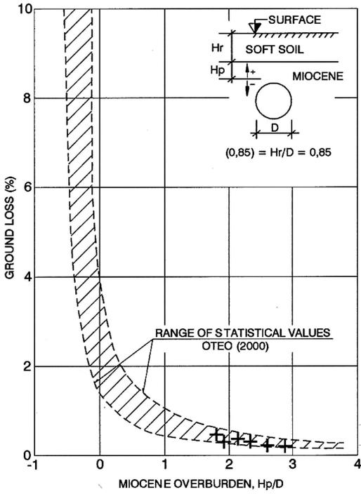
Figure 4. Ground loss measured in green filed trough.
