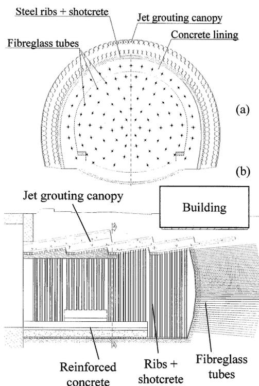
Figure 3. Construction details of jet-grouted canopy and face reinforcement (a) in cross-section and (b) longitudinally for the Florence tunnel (Russo and Modoni).
