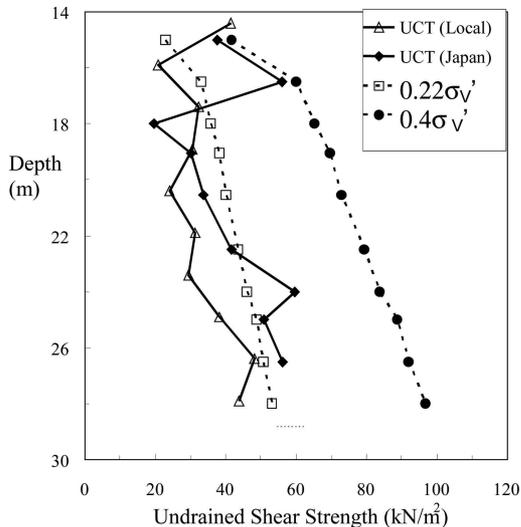
Figure 2. Effect of sampling method on undrained shear strength (UCT) for SAC clay.
