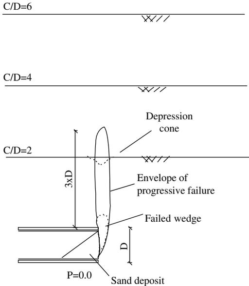
Figure 9. Sketches of tunnel geometry and failure development in PT series (Oblozinsky and Kuwano).
