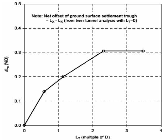
Figure 8. Relationship between net offset of ground surface settlement troughs ( $\Delta L_x$ ) at the plane strain conditions and lagging distance  $L_T$  in terms of multiple of tunnel diameter, D (Ng et al. 2004; Tang and Ng, 2005).
