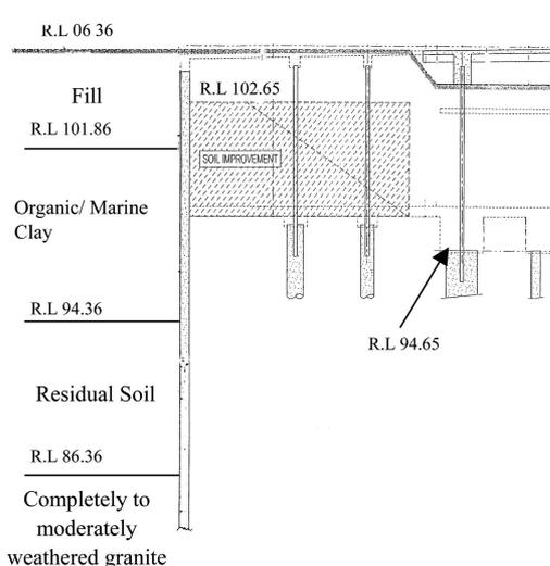
Figure 20. Use of deep soil mixing to provide an improved berm, HDB Centre at Toa Payoh.
