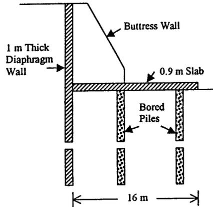
Figure 16. Configuration of permanent wall.
