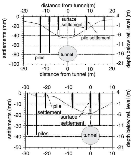
Figure 11. Surface and pile settlement at first (1st figure) and second (2nd figure) passage, (Kaalberg, et al., 2005).
