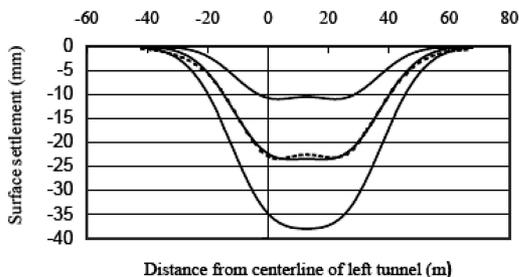
Figure 13. Comparisons of ground surface settlements for pillar width = 19 m, dashed and solid lines from numerical and empirical method, respectively (Rastbood et al.).
