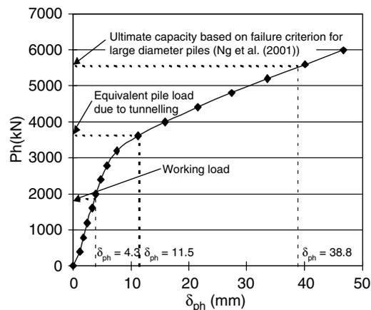
Figure 8. Pile head load versus pile head displacement (Lee et al., 2005).
