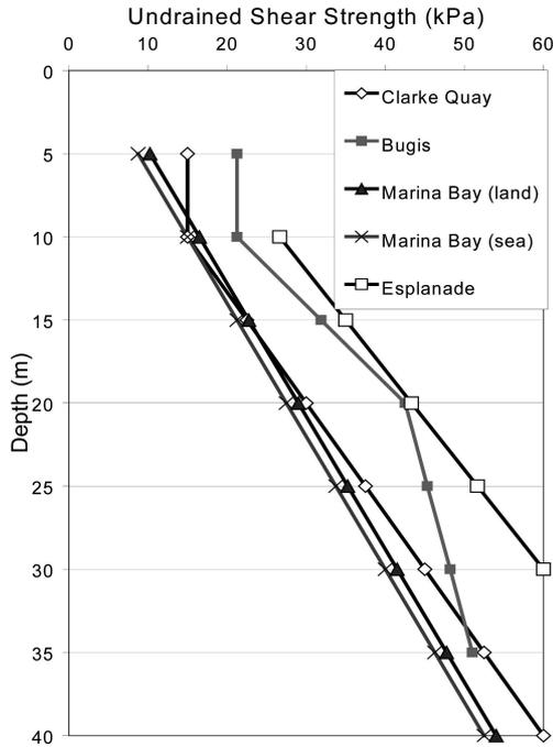
Figure 3. Undrained shear strength/depth profiles in the marine clay at various sites in Singapore, as used for design.
