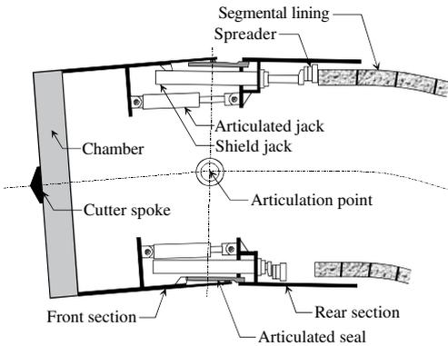
Figure 19. General feature of articulated shield (Sugimoto et al.).
