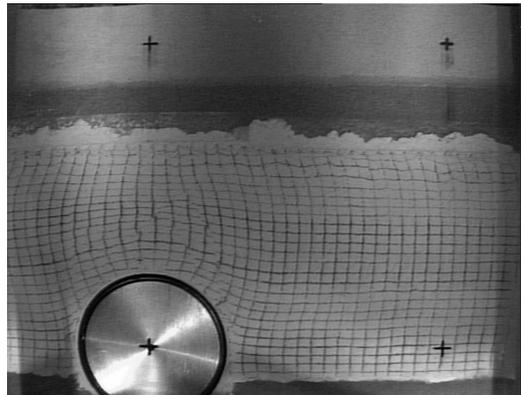
Figure 3. Deformation of clay at the end of consolidation after applying 55 kPa of sand in-flight (Pachen et al.).
