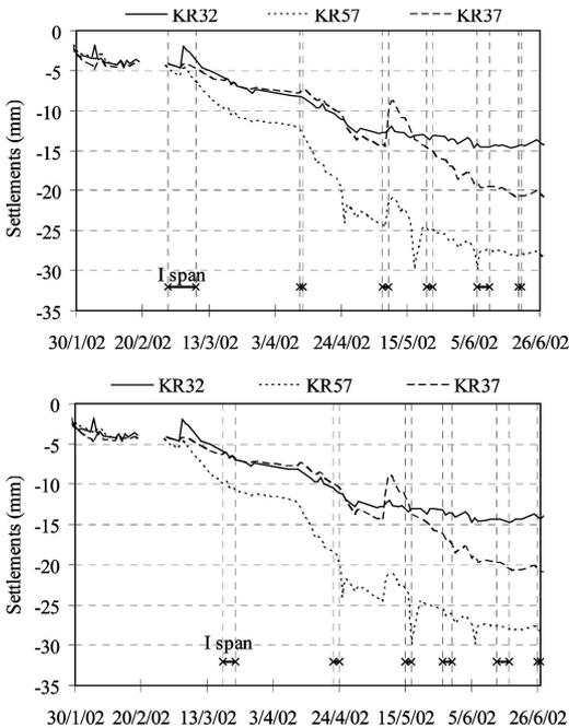
Figure 4. Settlements along a longitudinal section of the tunnel (left hand side) relating (a) to jet grouting operations and (b) excavation sequences (Russo and Modoni).
