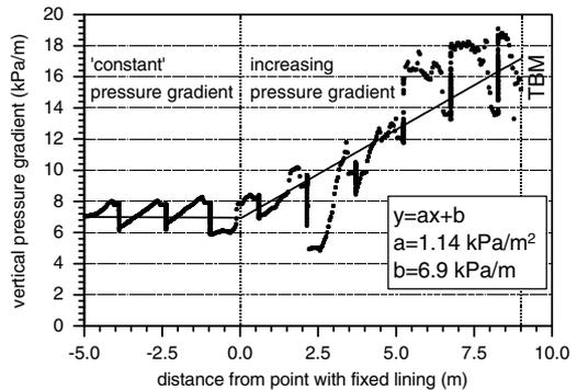
Figure 16. Example of gradient in the grout pressure as a function form the distance (0 on the X-axis represents the point where the lining is more or less fixed). The TBM is at 9 m). Results measured at Sophia Rail Tunnel (Bezuijen et al. 2004).
