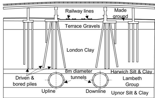
Figure 8. One of the piled bridge pier foundation case studies assessed during the CTRL project (*Jacobsz et al.*).
