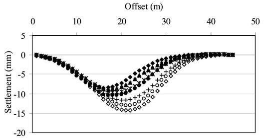
Figure 7. Data from the CTRL project showing settlements of an existing tunnel from tunnelling beneath it. The initial settlement profile is from the first Up-line tunnel, followed by developing profiles from Down-line tunnel (Moss and Bowers).
