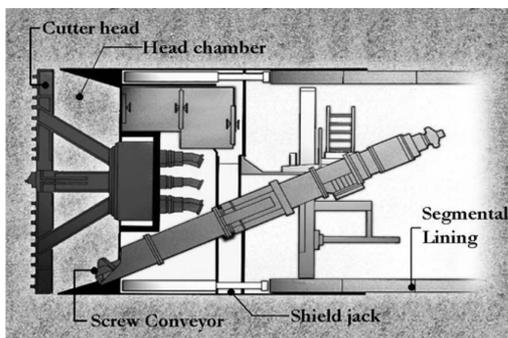
Figure 2. Schematic of typical EPB tunnelling machine.
