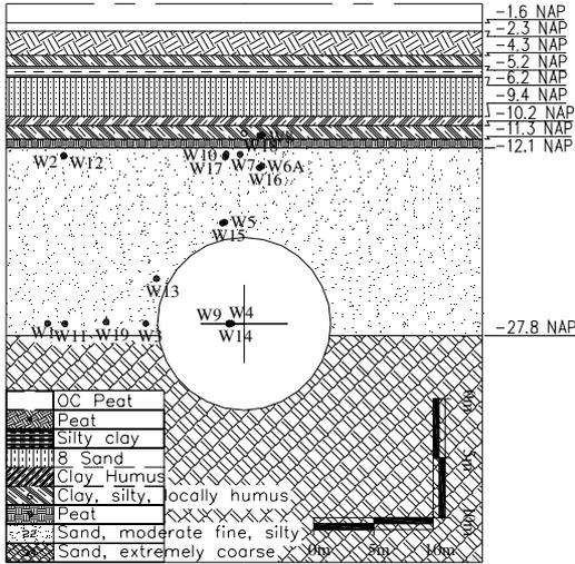
Figure 1. Geotechnical cross section at monitoring site (Autuori & Minec).
