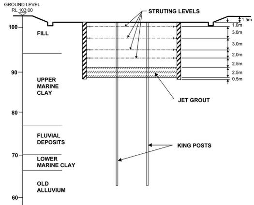
Figure 21. The excavation for the Central Services Tunnel (after Lim & Tan (2003)).
