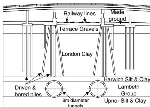
Figure 12. Cross-section Ripple Road Flyover, (Jacobsz et al., 2005).
