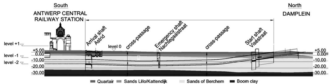
Figure 10. Longitudinal profile of the tunnel.
