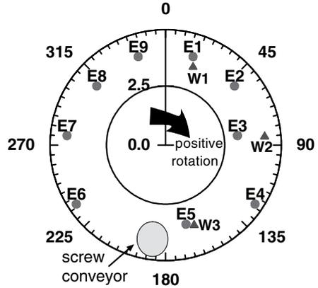
Figure 20. Position of instruments in the TBM looking from the tunnel to the TBM and definition of rotation (Bezuijen et al.).
