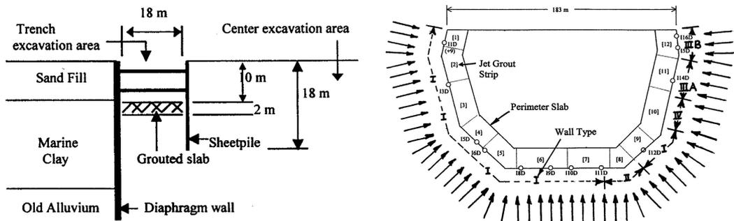
Figure 18. Perimeter concrete slab (16 m wide and 0.9 m thick) at formation level acting as a compression ring.
