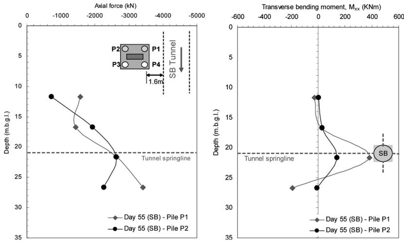
Figure 11. Response of pile foundation in terms of axial force and bending moment (Pang *et al.*).
