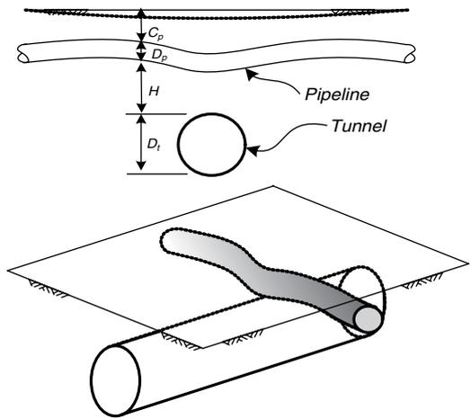
Figure 4. Schematic representation of the problem (Vorster et al.).
