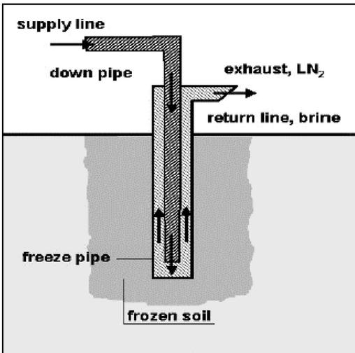
Figure 9. Ground freezing principle.
