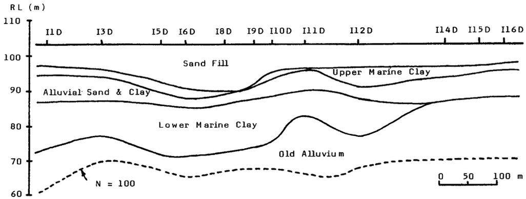
Figure 17. Soil profile along the perimeter of excavation from south to north (Section A-A').
