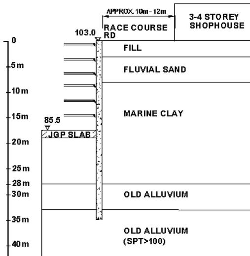
Figure 10. Jet grout slab used as a buried strut, cut-and-cover tunnels along Race Course Road.
