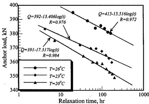
Figure 13. Results from a relaxation load test, with head load locked off at 400 kN, for the 3 m long anchor (Tamano *et al.*).
