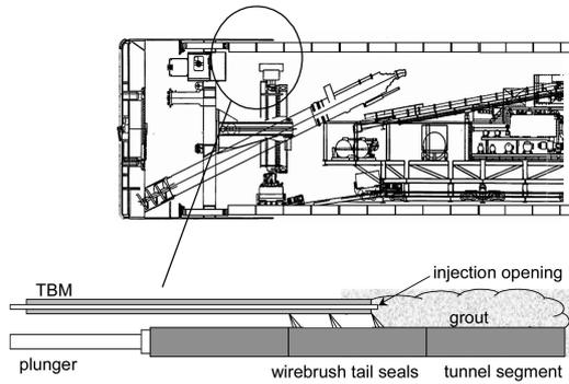
Figure 15. Sketch of TBM and details of injection system (Bezuijen and Talmon).
