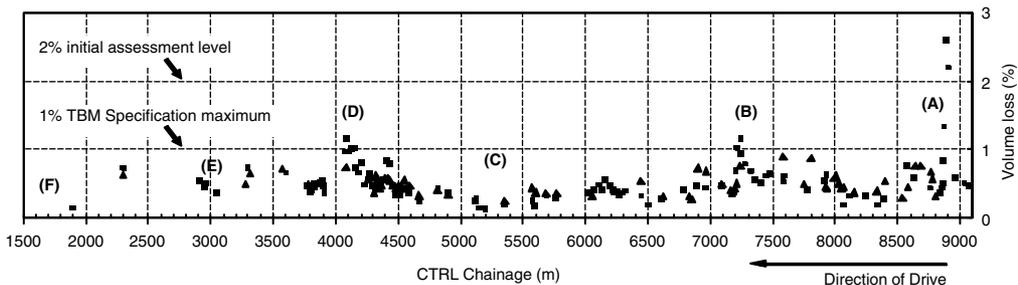
Figure 5. Volume losses for the upline (square symbols) and downline (triangles) tunnel drive on Contract 220 of the CTRL project (Bowers and Moss).
