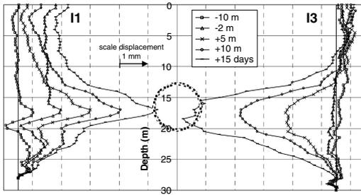
Figure 6. Transverse horizontal movements either side of tunnel from Toulouse Metro project (Vanoudheusden *et al.*).
