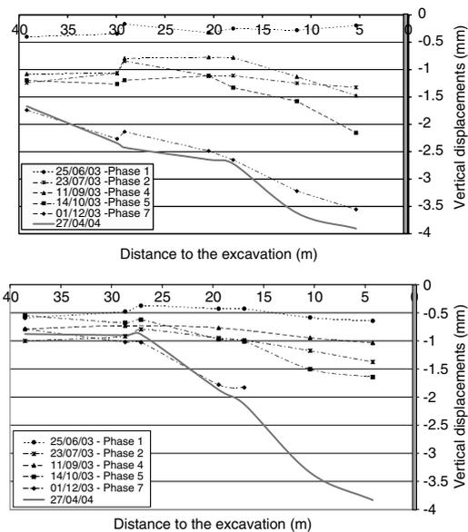
Figure 14. Settlement profiles along monitoring sections perpendicular to the excavation (a) greenfield case and (b) along the instrumented buildings (Emeriault *et al.*).
