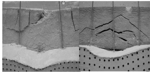
Figure 3. Failure mechanism of the weak (left) and the strong wall (right), (Carporaletti et al., 2005).
