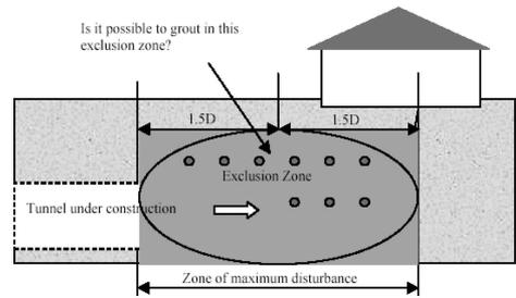
Figure 2. Grouting in exclusion zone in compensation grouting.
