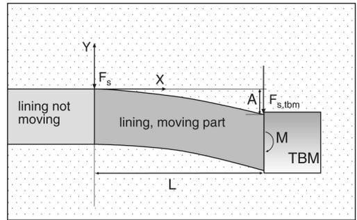
Figure 8. Idealised behaviour of tunnel lining showing flotation in fluid grout (Bezuijen and Talmon, 2005).
