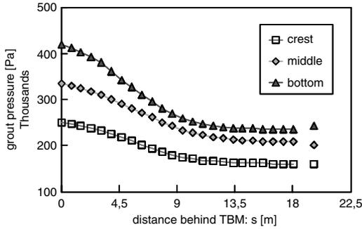
Figure 18. Calculated grout pressure for Sophia Rail Tunnel as a function of the distance behind the TBM (Talmon and Bezuijen).
