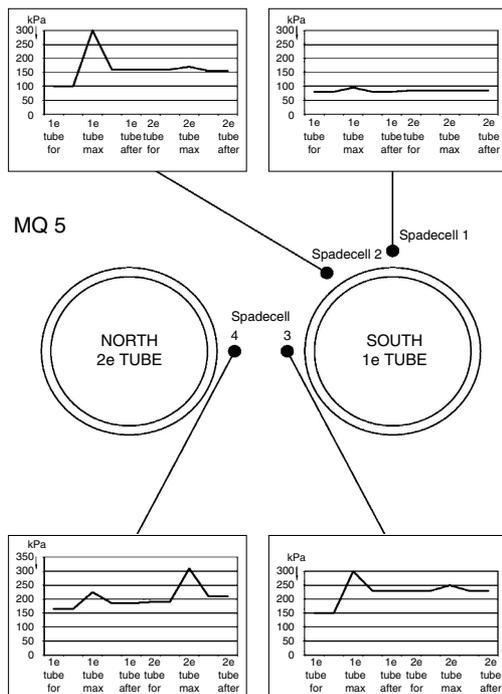
Figure 9. Results of spade cells (in kPa), (Kwast, E.A. & G.P.C. van Oosterhout, 2005).
