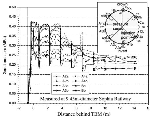
Figure 17. Results of field measurement on the grout pressure at Sophia Rail Tunnel (Bezuijen et al. 2004).
