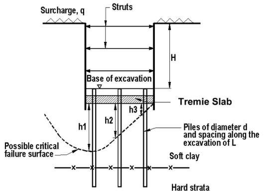
Figure 9. Basis for the estimation of uplift pressures on the tremie slab, Marina Bay Station.
