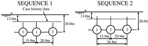
Figure 6. Construction sequence and geometry of triple tunnels (Chapman et al.).
