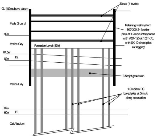
Figure 13. An example of a 'floating' wall system, used for part of the KPE construction.
