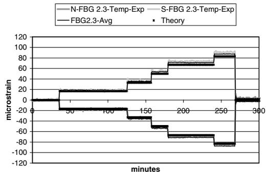
Figure 2. Comparisons between measured and theoretically calculated strains at one FBG location resulting from vertically-induced movement of the Smart Rod in 0.5 mm increments. (Metje *et al.*).
