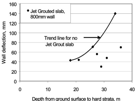
Figure 11. A comparison between the recorded deflections for 17.5 to 18 m deep excavations, with and without a single jet grout slab just below the base of the excavation.
