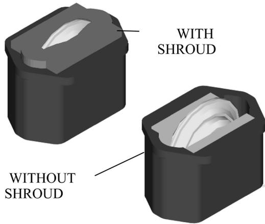
Figure 14. Shape of the disc cutter.
