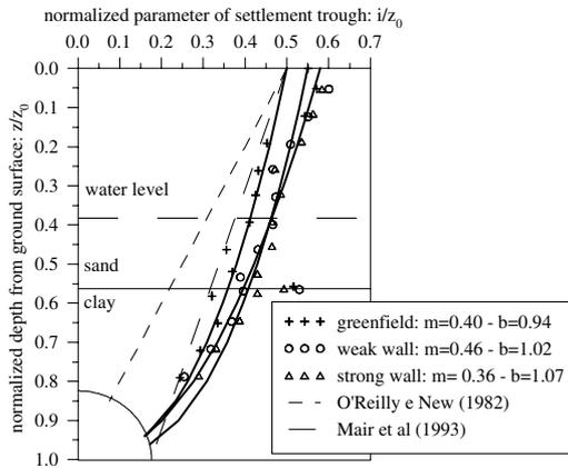
Figure 2. Normalized parameter of settlement trough ( $i/z_0$ ) against normalized depth from ground surface ( $z/z_0$ ), (Carporaletti et al., 2005).
