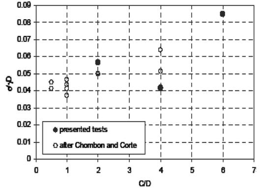
Figure 10. Normalised supporting pressure at failure against C/D ratio (Oblozinsky and Kuwano).
