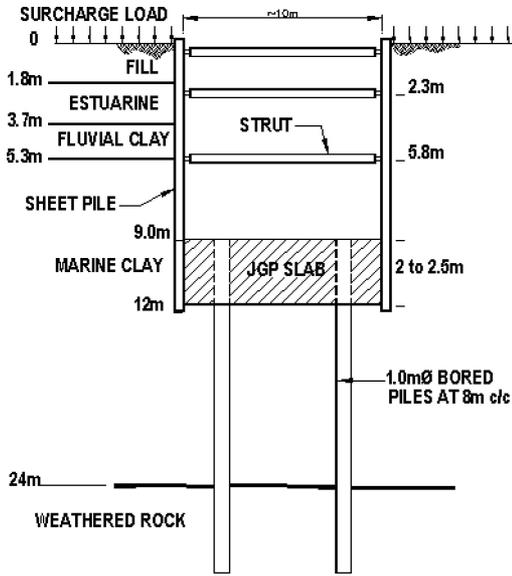
Figure 12. The 'floating' retaining system, Entrances 1 and 2, Clarke Quay Station.
