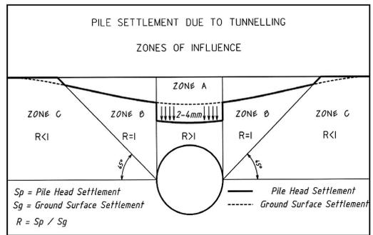
Figure 9. Zones of influence of piled settlement due to EPB shield tunnelling in London Clay (Selemetas *et al.*).
