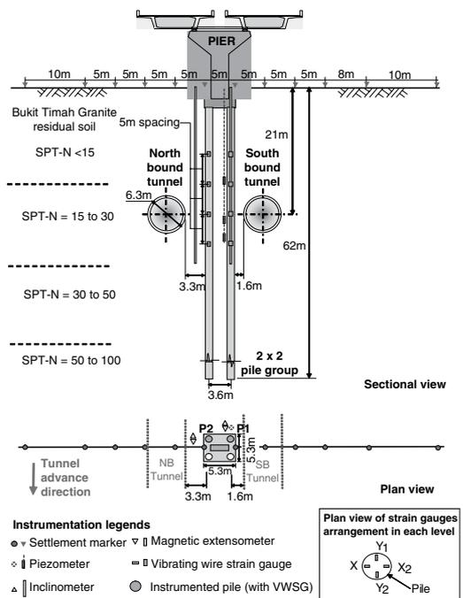
Figure 10. Typical section and instrumentation layout for pile-tunnel interaction study reported by Pang *et al.*
