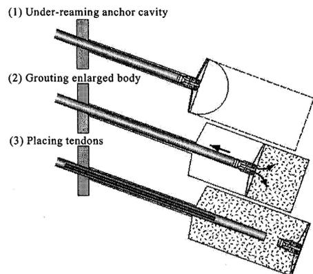
Figure 12. Construction sequence for splits anchors (Tamano *et al.*).
