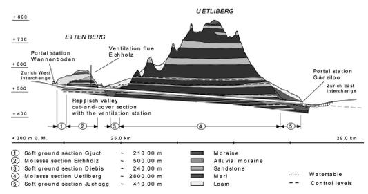
Figure 6. Longitudinal profile along the tunnel.
