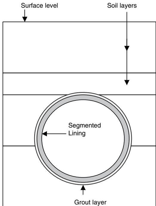
Figure 21. Schematic representation of the tunnel section modelled (Lokhorst et al.).
