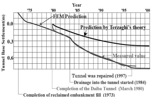
Figure 14. Comparison between the measured and computed values at the Daiba Eastbound tunnel (Komiya et al.).
