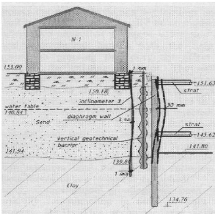
Figure 13. Excavation profile near building N1.
