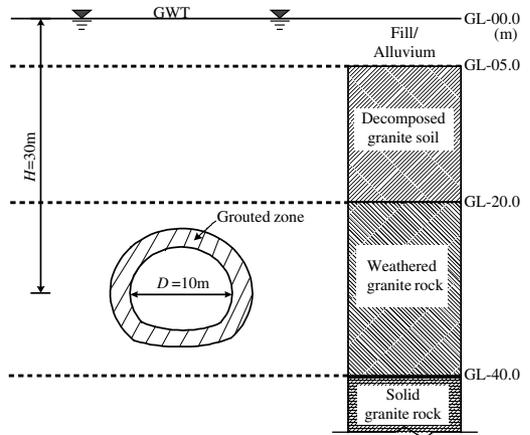
Figure 2. Ground profile for tunnelling condition analyzed (Yoo & Kim).
