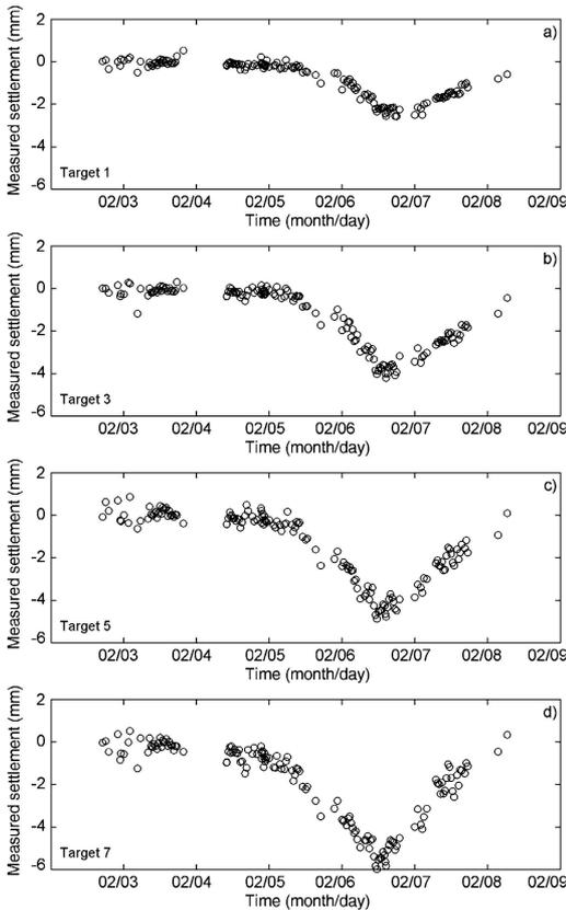
Figure 1. Results from real-time monitoring using image analysis techniques described by Take *et al.* (note that the targets are at increasing distances from camera: 1 the nearest and 7 the furthest away).
