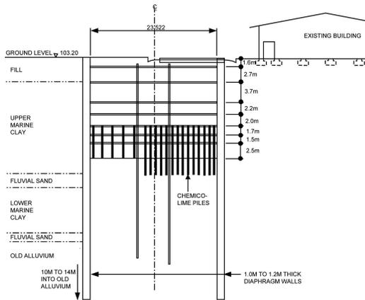
Figure 6. The excavation support system for Bugis Station.
