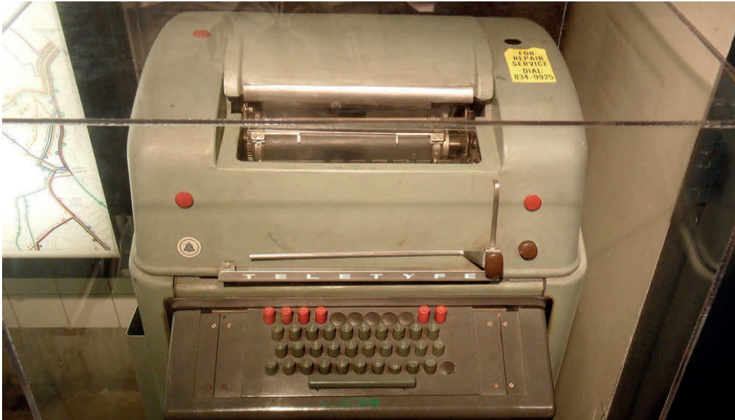
Figure 1.6: A teletype unit, similar to the one that would have been used with the ENIAC ( Eric Fischer CCBY2.0 ).
