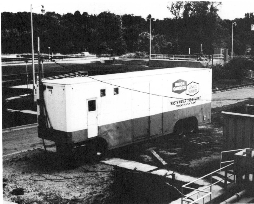
FIGURE 6. Typical mobile UNOX ® pilot plant unit used for conducting on-site pilot plant tests. (Courtesy of Union Carbide Corporation.)
