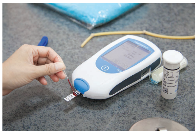
FIGURE 2.1 CoaguCheck System™ including testing, lancing device, and test strips.
