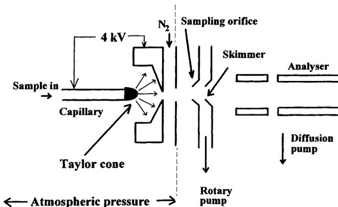
Figure 1.7 Schematic diagram of an electrospray ionisation source
