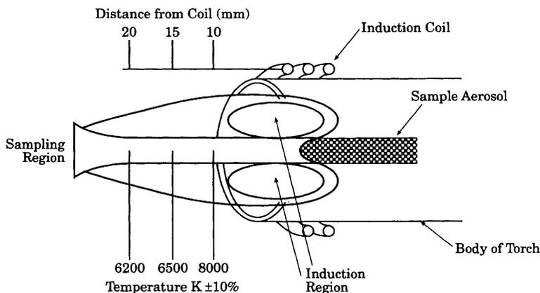
**Figure 1.12** Schematic diagram of an ICP/MS ion source (Redrawn from a diagram supplied by VG Elemental, with permission)
