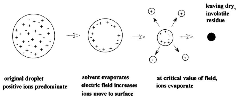
Figure 1.6 Schematic representation of the electrospray ionisation process
