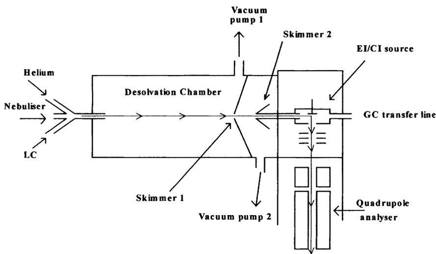
Figure 1.4 Schematic diagram of a particle beam LC/MS interface
