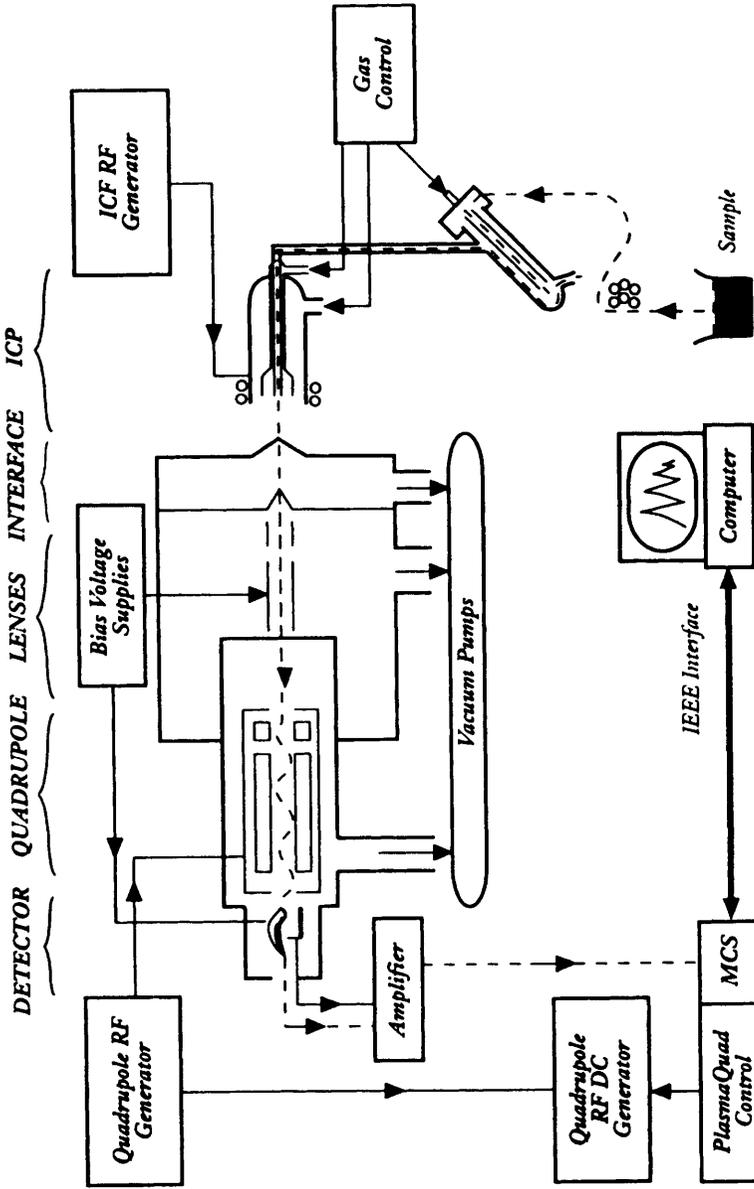
Figure 1.13 Schematic diagram of an VG PlasmaQuad ICP/MS instrument (Reproduced from material supplied by VG Elemental)
