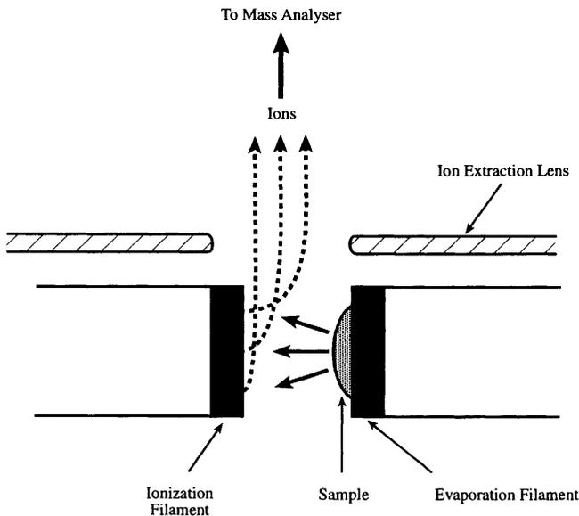
**Figure 1.11** Schematic diagram of a double-filament thermal ionisation source
