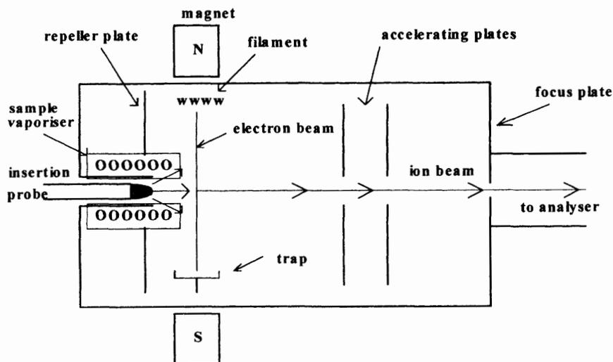
Figure 1.2 Schematic diagram of an Electron Ionisation source
