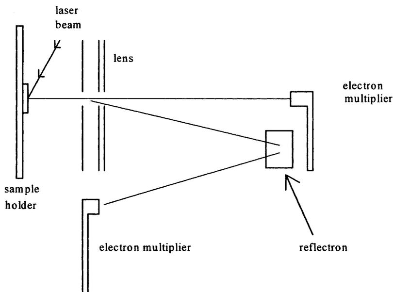
**Figure 1.9** Schematic representation of the MALDI-TOF mass spectrometer (reflectron type)
