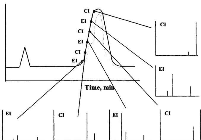
**Figure 1.5** *A schematic representation of alternate Chemical Ionisation/Electron Ionisation*
