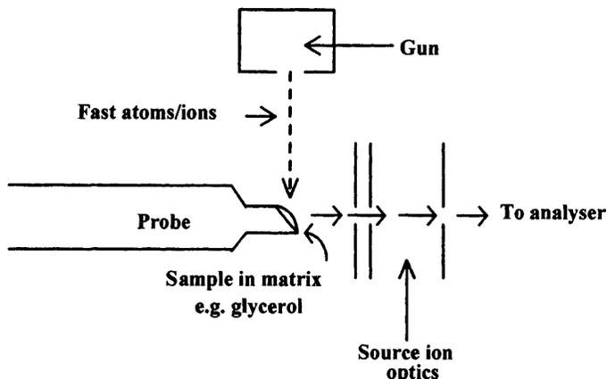
**Figure 1.10** Schematic representation of a FAB/LSIMS ion source
