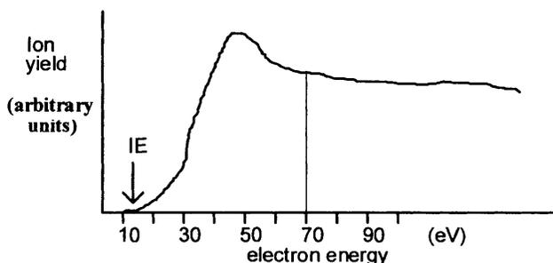
**Figure 1.3** Typical variation in ion yield from an organic compound with increasing electron beam energy
