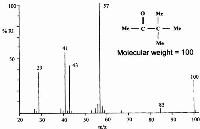
Figure 1.1 Electron ionisation mass spectrum of methyl t-butyl ketone
