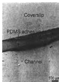
Figure 2. A sealed channel. Figure 3. Etch rate vs. (a) HF concentration and (b) HF flow rate.
