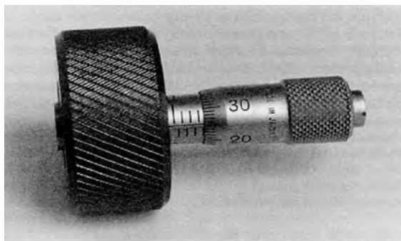
Figure 1.5 Micrometer screw gauge adapted for measuring the anode-to-sample gap 1 (Reproduced with permission from John Wiley & Sons)
