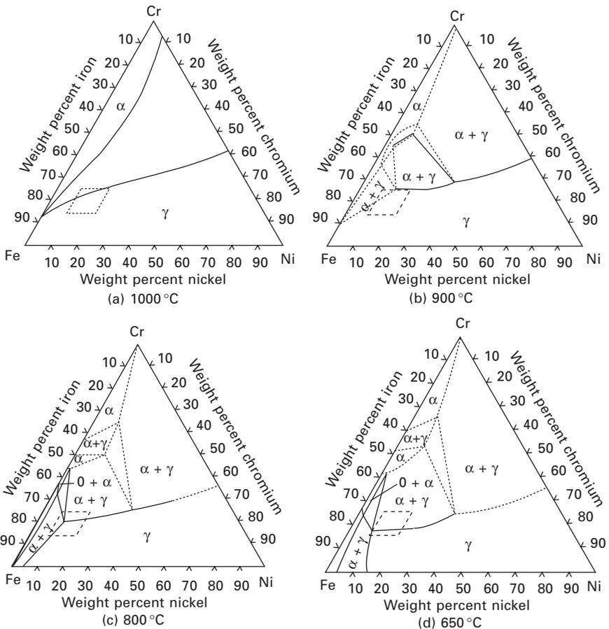
1.3 Isothermal sections of the Fe–Ni–Cr ternary system shown at various temperatures. The small boxes (dotted lines) represent the typical range of Ni (~ 8–20 wt%) and Cr (~ 15–25 wt%) concentrations found in many commercially austenitic stainless steels.
