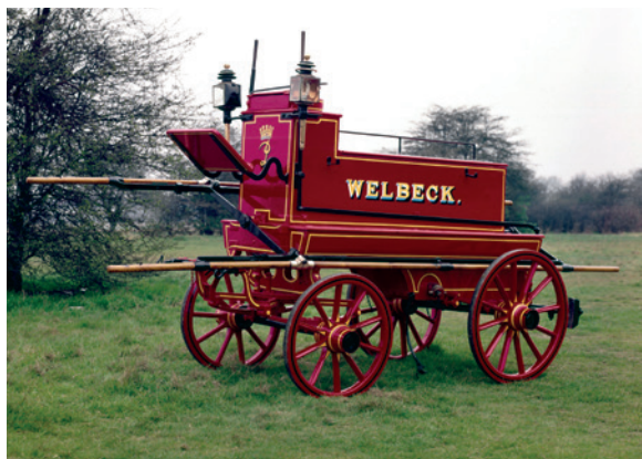
Horse-drawn manual pump built by Merryweather and Sons in 1866. With twenty-two men to work it the engine could deliver 100 gallons of water per minute to a height of 120 feet. This example was purchased by the Duke of Portland for his Welbeck Abbey Estate.
