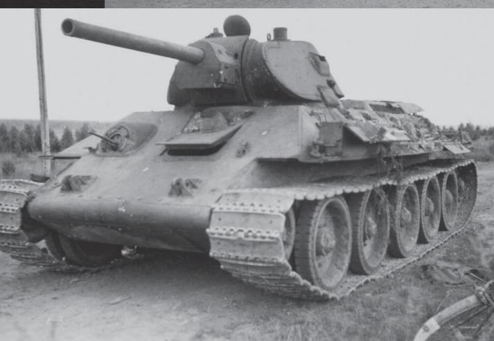
The T-34 was a nastv surprise for the German troops invading the Soviet Union. The sloping armour offered good protection against most German weapons. The powerful long-barrelled 7.62cm F-34 gun proved to be a formidable weapon able to deal with all German tanks. The T-34 had a good power-to-weight ratio and wide tracks made it much more mobile than any other tank then in service. (Anderson)
