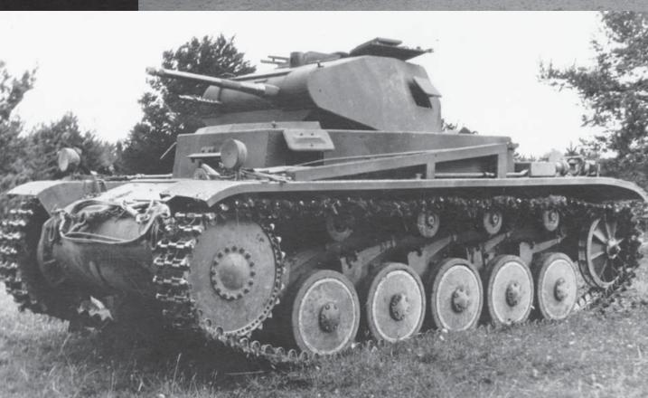
The PzKpfw II was lightly armoured and mounted a 2cm KwK 30 cannon but was effectively used to attack and defeat enemy infantry positions. Although obsolete, it was still being used in 1944 as an escort tank in *Panzer-Begleit-Kompanien* (Tank Support Company) of the *Heeres-StuG-Brigaden* (Assault Gun Brigade). (Münch)
