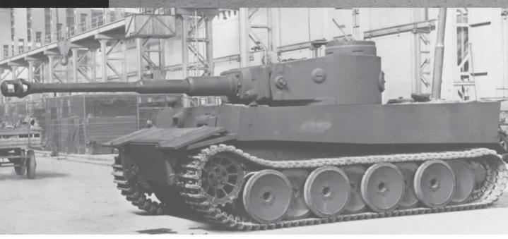
A pre-production PzKpfw VI Tiger (H) in the Henschel factory. The vehicle is fitted with an additional armour plate (not used on production tanks) which was lowered to provide extra protection for both the front plate and drive sprockets. The vehicle is still to be fitted with track guards and tools. (Tank Museum)
