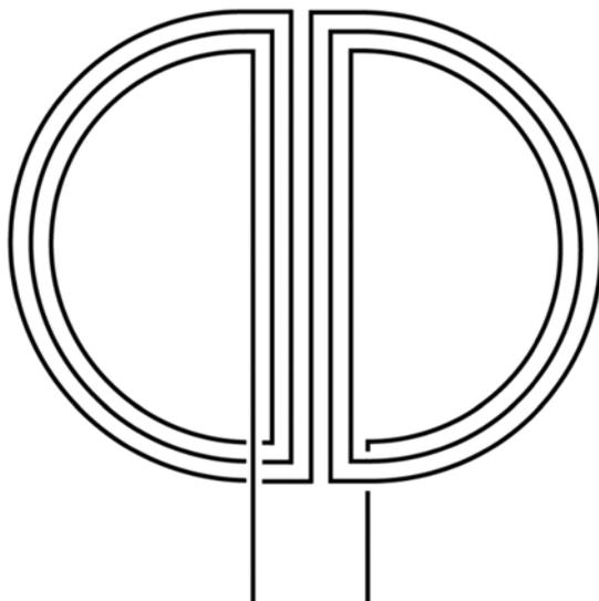
**Figure 1.4** Schematic of a flat gradiometer coil used in Earth's field NMR that is sensitive to a flat region parallel to the plane of the coil. Coils with length scales from 61 cm to 6 m have been used to detect proton signals from water without pre-polarization.
