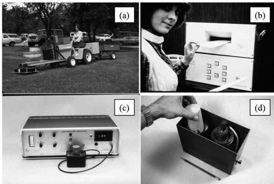
**Figure 1.1** (a) Photo of a mine detector that is mounted in front of a tractor. The trailer carried the batteries. (b) Photo of a mail bomb detector based on  $^{14}\text{N}$  nuclear quadrupole resonance (NQR). NQR is well-suited for mobile instrumentation because it requires no magnetic fields. (c) Photo of a soil moisture detector and (d) photo of a cement core moisture detector probe, presaging the modern rock core analyzers, such as those described in Chapter 10.
