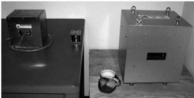
**Figure 1.3** Three 1 T permanent NdFeB-based magnets with 40, 25, and 5 mm gaps. The first two were made by Neomax (Japan) and the third by Aster Enterprises in the US.
