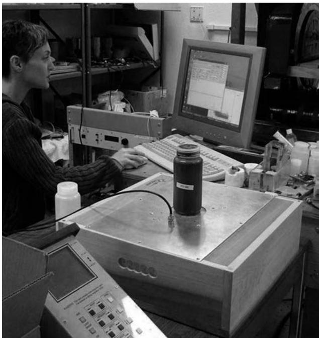
**Figure 1.2** Unilateral NMR device with which a signal is obtained from a sample of crude oil in a 500 mL plastic bottle on top of the device.
