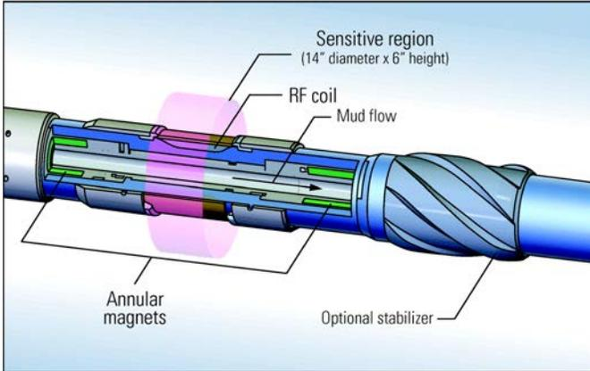
**Figure 2.1** Schematic view of the NMR logging-while-drilling device with an azimuthally symmetric sensitive region described in ref. 13. The two permanent magnets, shown in green, are magnetized along the tool axis in opposite directions and generate a magnetic field that is radial in the sensitive region. Illustration copyright Schlumberger. Used with permission.
