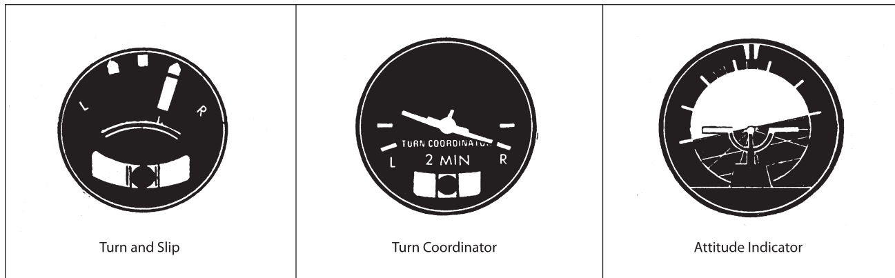
Figure 3-21. The turn and slip, turn coordinator, and attitude indicator indications in a standard-rate turn at 100K. Setting up the thumb rule for the bank angle only works for the balanced turn (no slip or skid).
