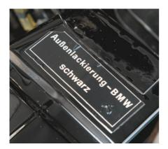
The paint colour sticker on the inner wing always had the name of the paint without a capital letter. "Außenlackierung" means "exterior paint". Note the bubbles and imperfections in the way this original sticker was applied.
