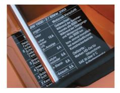
Partly concealed by the bonnet catch operating rod, this sticker combines the list of fuses and their functions on an early six-fuse car with recommendations for engine oil types and oil change intervals.
