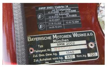
Yet another type of European conformity sticker is seen here, this time showing different code numbers for cars with manual transmission (Schaltgetriebe) and automatic transmission. The red paint which has found its way into the stamped chassis number (2795096) is incorrect and was probably deposited there during some repainting work.
