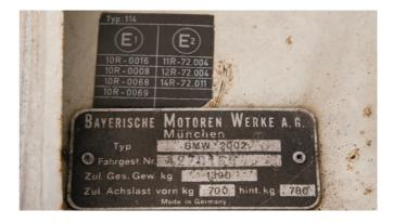
The chassis number plate on this earlier 2002, numbered 4 270 155, has the same format as the later type. However, the European conformity sticker is very different. The number 114 at the top was BMW's type code for the 2002.
