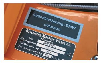
Reproduction chassis plates and paint colour stickers have been available for some time through specialist dealers. On this chassis plate, note the incorrect size and spacing of the figures in the chassis number and the cross-head fixing screws instead of rivets. The configuration of the paint sticker is worth comparing with the original example shown on page 14.
