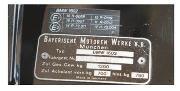
The chassis number or VIN plate was always attached to the inner front wing by rivets. This example is on a late 1602. The chassis number itself is stamped into the unprinted section in the middle: BMW expressed the numbers as a single block (in this case, 3562264), but in this book we have divided the numbers into three blocks for clarity (e.g., 3 562 264). Above the plate is the European conformity sticker.
