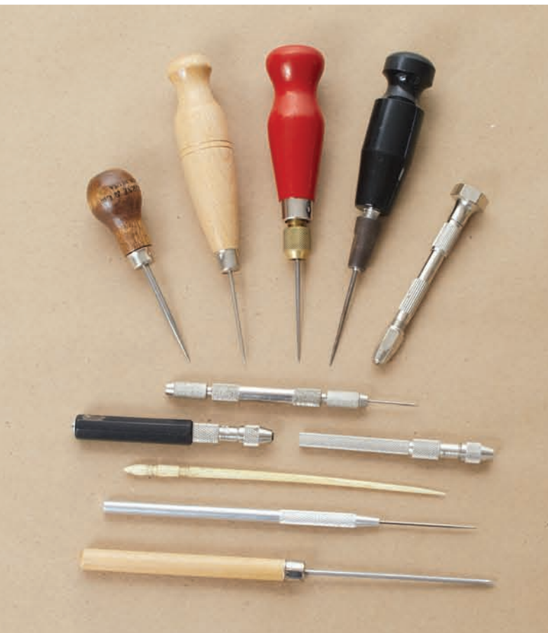
A selection of awls, most often used for punching holes
