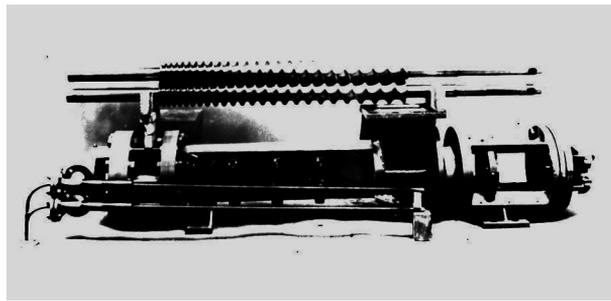
**Figure 1.31** Pioneering screw, circa 1955, with degressive pitch
