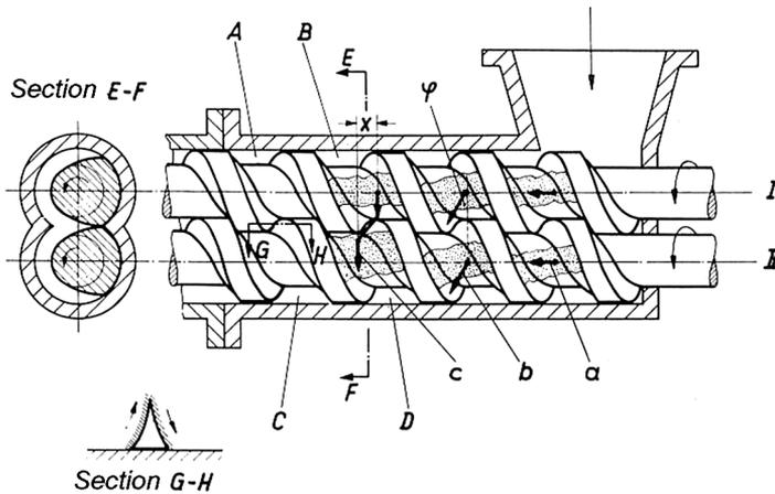
**Figure 1.22** Multiple shaft co-rotating extruder system with full intermeshing and mutual cleaning of the shafts. There is a continuous connection between A, B, C, and D, etc. The possible material movements in principle are as follows:
