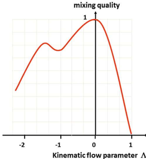
**Figure 1.60** Influence of the kinematic parameter of flow  $\Lambda$  on the mixing quality [11]
