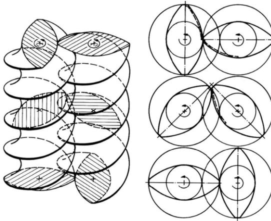
**Figure 1.26** Practical limit for double-flighted elements
