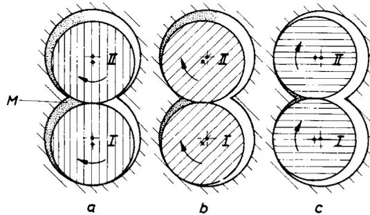
**Figure 1.24** Operating method of eccentric, synchronous, co-rotating, circular discs: *a, b, c* three operating positions: mass *M* is crushed and sheared in the key during the quarter turn around their rotation axis described by each disc (*I* and *II*).
