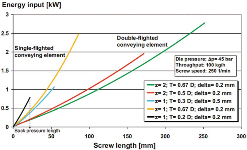
Figure 1.65 Energy input in the pressure build-up zone for different conveying elements
