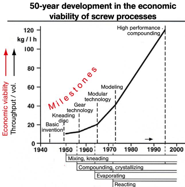
**Figure 1.48** Dynamic development of the co-rotating extruders
