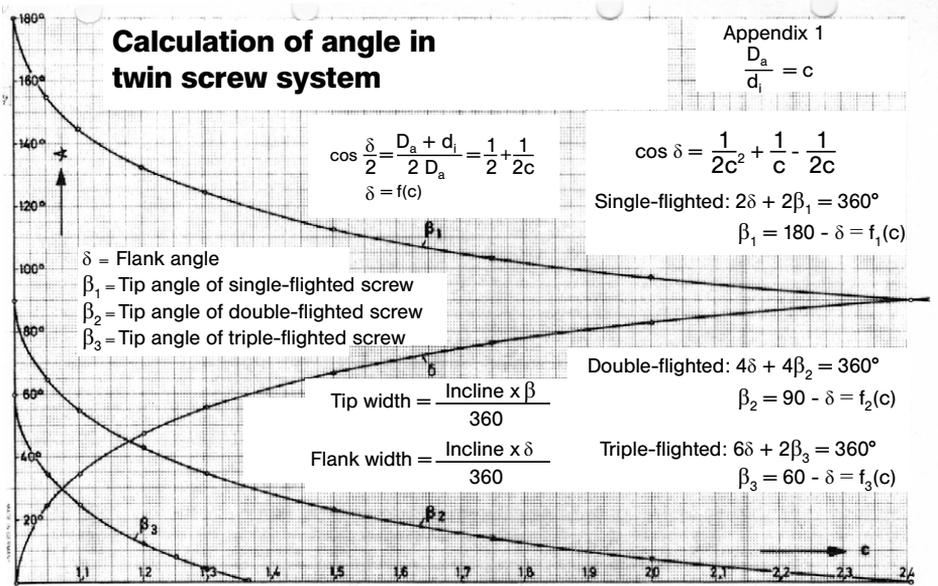
Figure 1.18 Characteristic angle diagram [11]
