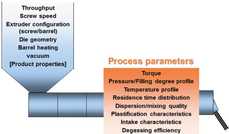
**Figure 1.52** Parameters of the compounding process
