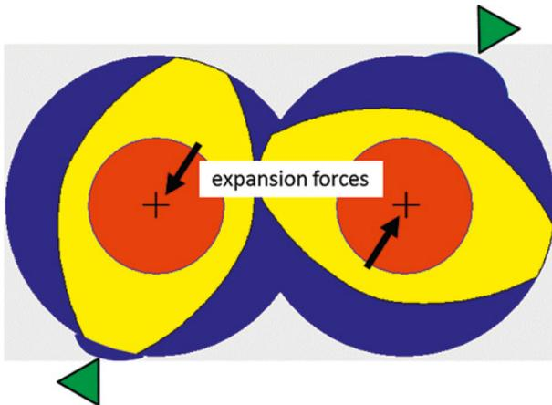
**Figure 1.58** Cylinder wear caused by expansion forces [5]
