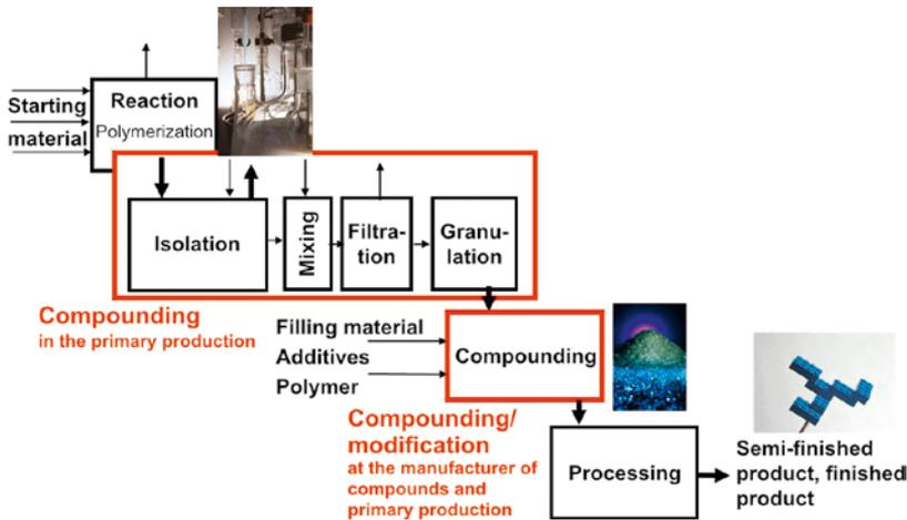
**Figure 1.2** Plastic production with the compounding steps at the producer of raw materials and manufacturer of compounds
