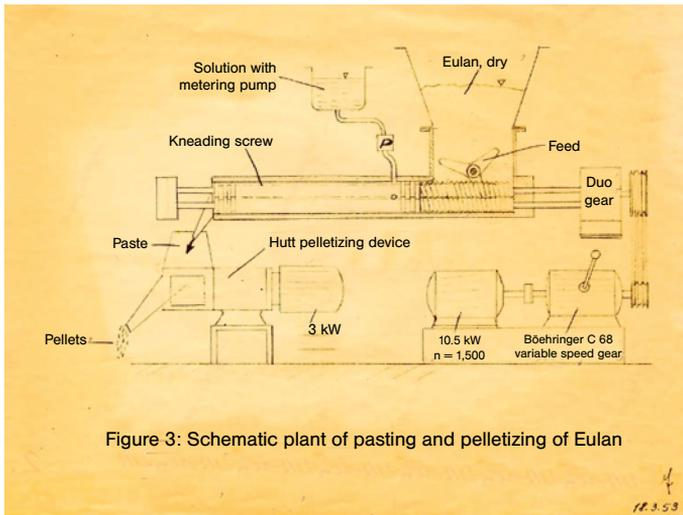
Figure 3: Schematic plant of pasting and pelletizing of Eulan
