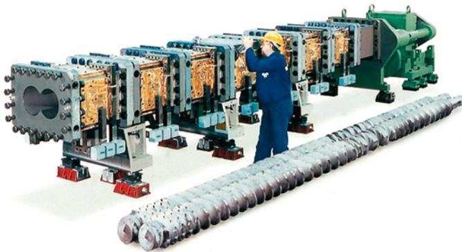
**Figure 1.46** Large co-rotating extruder: Megacompounder ZSK 340 (Courtesy: Werner & Pfleiderer)
