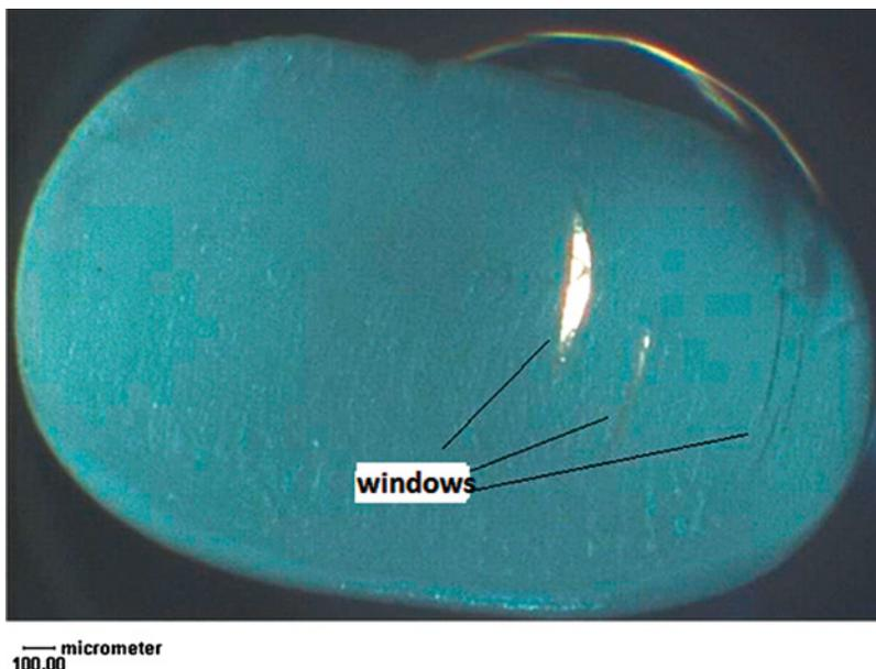
**Figure 1.53** Unplasticized particles (so-called windows) within a pellet
