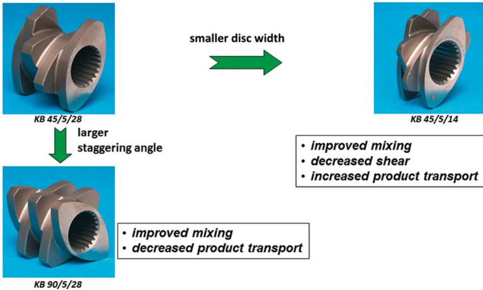
**Figure 1.55** Geometric values and process variables of a double-flighted kneading block
