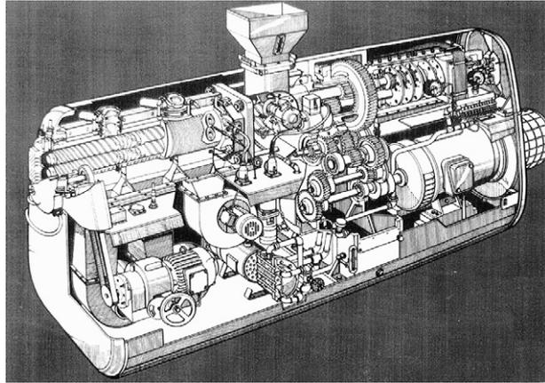
**Figure 1.8** Section through a historic ZSK (Coperion GmbH)
