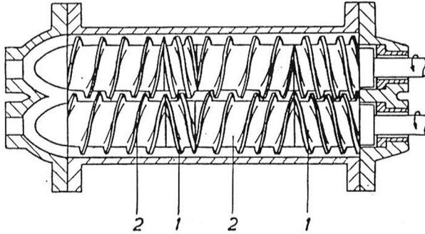
**Figure 1.30** “Backward pumping screw” with left/right hand thread
