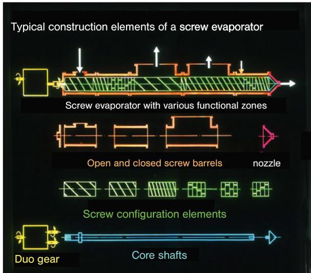
**Figure 1.45** Overall machine comprising typical modular components
