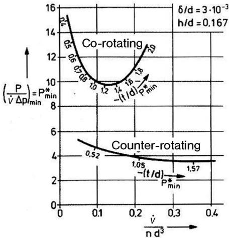
Figure 1.40 Energetic optimization, i.e., “minimal stress” for co-rotating and counter-rotating screws
