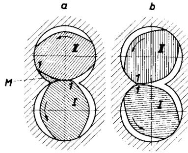
**Figure 1.25** Double-flighted kneading discs operation of blunted lens-shaped discs
