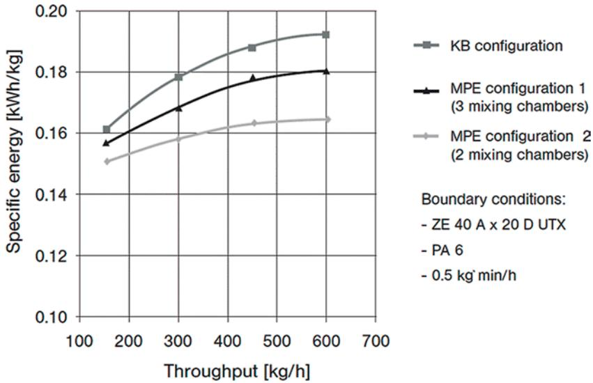
**Figure 1.57** Energy input as a function of throughput for polyamide melting with kneading block and MPE plastification zones [10]
