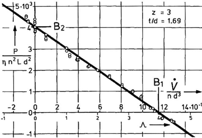
Figure 1.39 Power measurements on a co-rotating extruder
