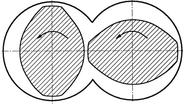
**Figure 1.16** Screw with tip width, cross-section
