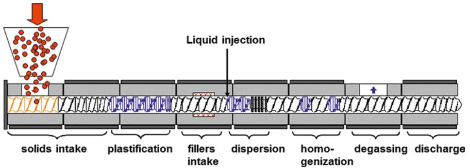
**Figure 1.51** Processing zones of a twin-screw extruder
