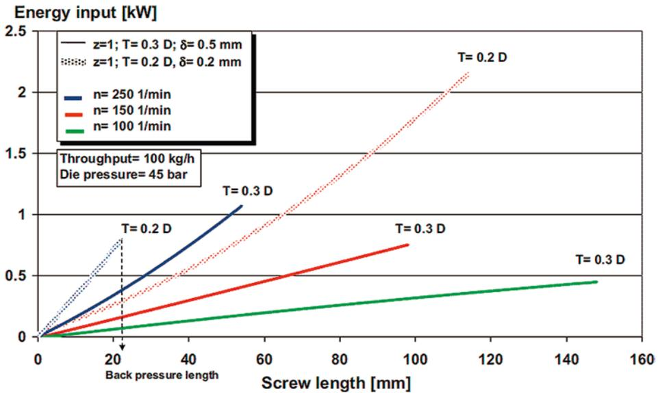
Figure 1.66 Influence of screw speed and pitch on the energy input in the pressure build-up zone
