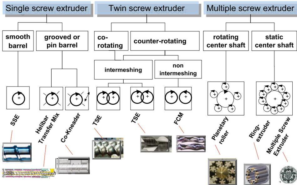
**Figure 1.4** Classification of screw machines/extruders by the number of shafts
