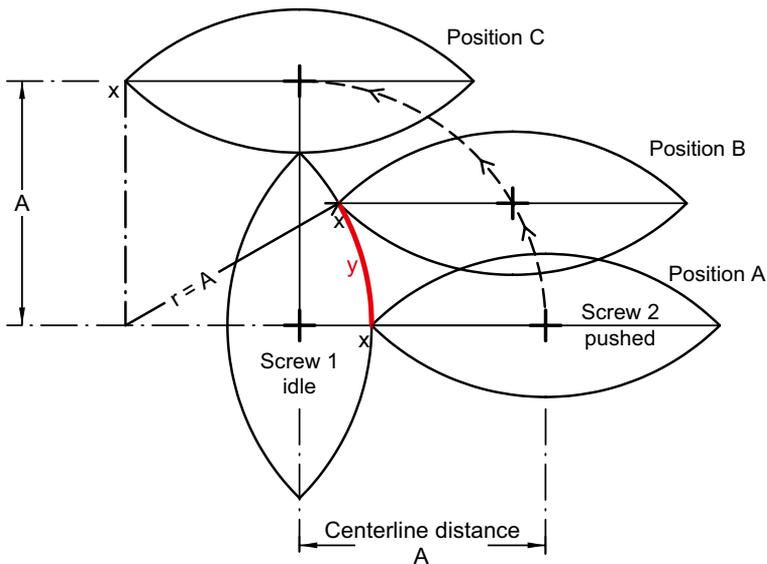
**Figure 1.15** Kinematic equivalent view “movement without rotation” (screw with tip width 0)
