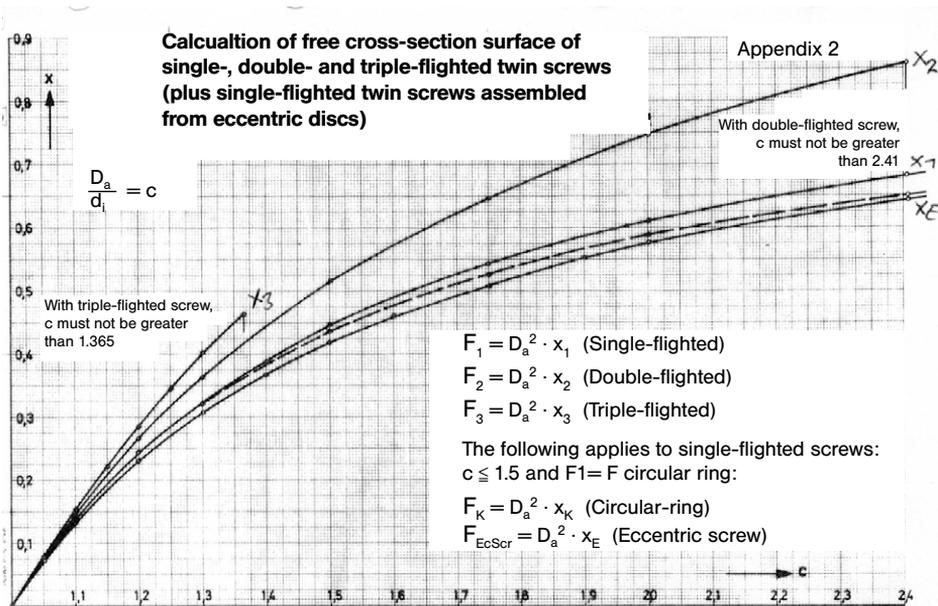
Figure 1.19 Characteristic cross-section area diagram [11]
