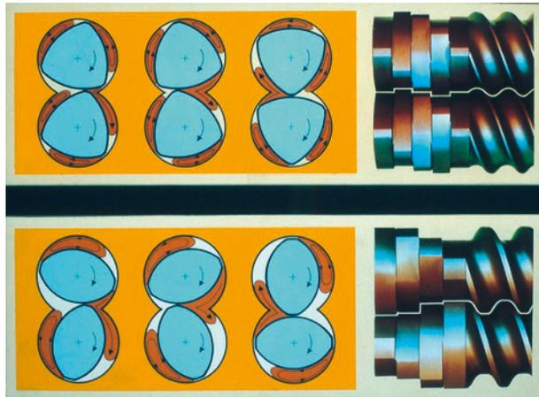
**Figure 1.44** Modular technology in screws (Courtesy: Werner & Pfleiderer)
