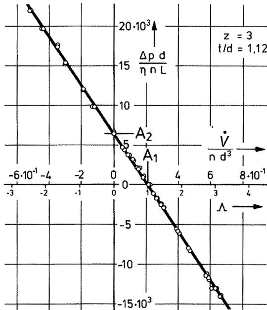
**Figure 1.38** Pressure measurements on a co-rotating extruder
