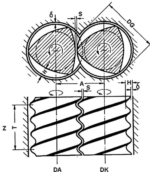
**Figure 1.42** Internal geometry of the co-rotating extruder with dimensioning
