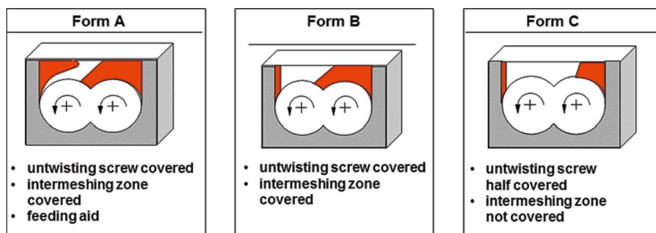
**Figure 1.64** Vent inserts (according to Coperion [13])
