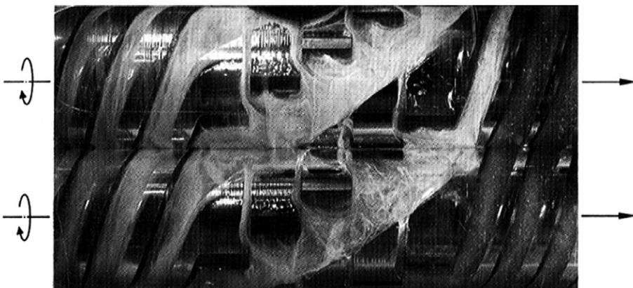
**Figure 1.56** Melt streams in a kneading block zone: broad main stream in the feed direction and narrow leakage flow [9]
