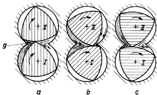
**Figure 1.27** Operating method of 3-point kneading discs:  $a$ ,  $b$ ,  $c$  three operating positions.
