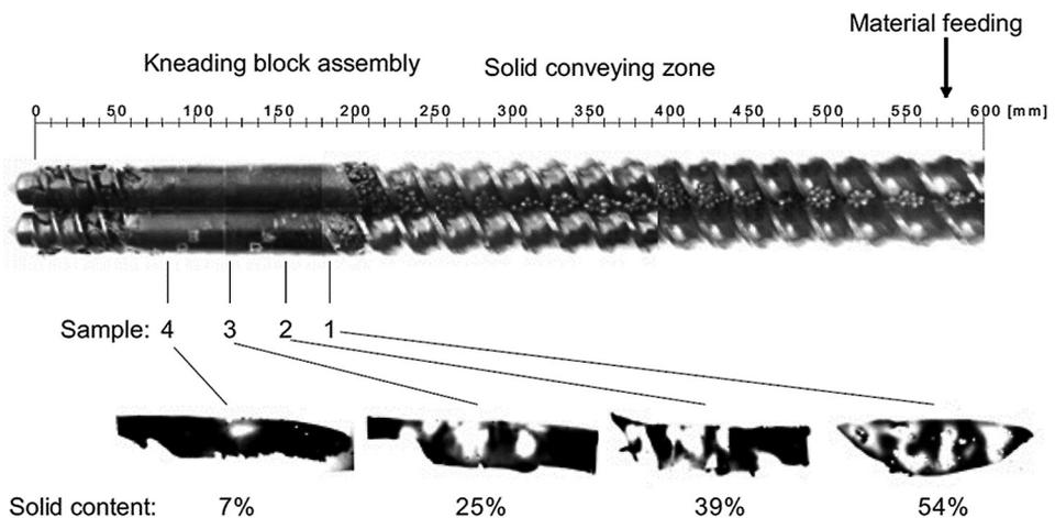
**Figure 1.54** Melting profile along a plastification zone [7]
