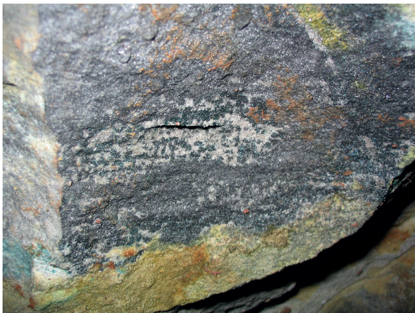
Plate 9. Coarse-grained sandstone from Alderley Edge containing disseminated grey to black copper and lead sulphide ores, with minor alteration to yellow and blue supergene minerals. This type of ore is typical of the Triassic sandstones at the locality.
