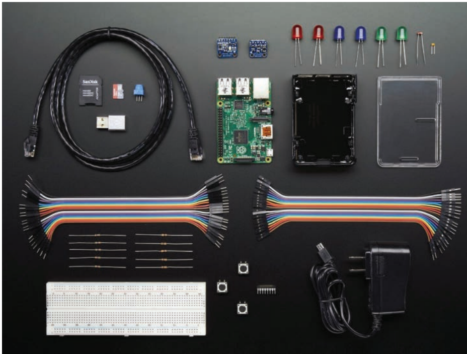
FIGURE 2-7 Contents of the Starter Pack for Windows 10 IoT Core on Raspberry Pi 2. A pack containing Raspberry Pi 3 is very similar. Source: http://www.adafruit.com .
