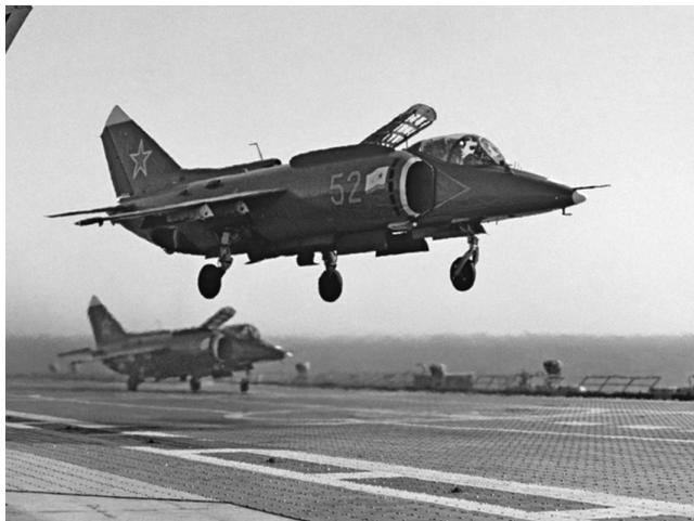
**FIGURE 1.1** Yak-38 fighter, where alloy 1420 was used (first serial utilization of the Al–Li alloy).
