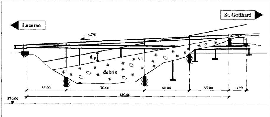
Fig. 3. Longitudinal section through the Reuss bridge A2 Wattingen (uphill track ROMEO)
