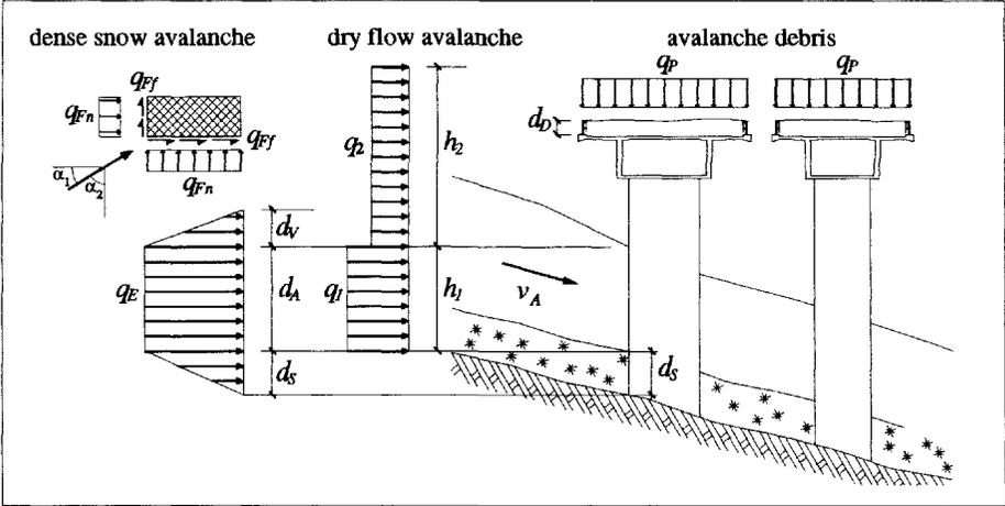
Fig. 2. Actions on piers and girders of the Reuss bridges A2 Wattingen, normal and accidental event
