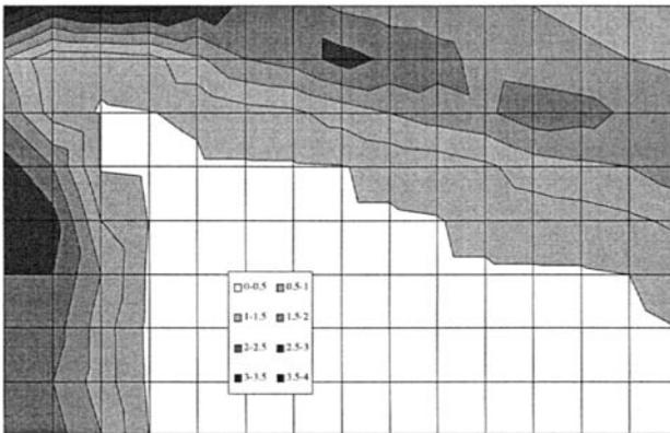
Fig. 2. Results obtained by BBRI using a numerical model to determine the pressure distribution at the upwind corner of the rooftop of a building.
