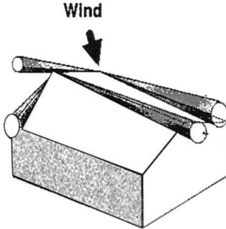
Fig. 1. Delta-wing vortex pairs on duopitch roof [11].
