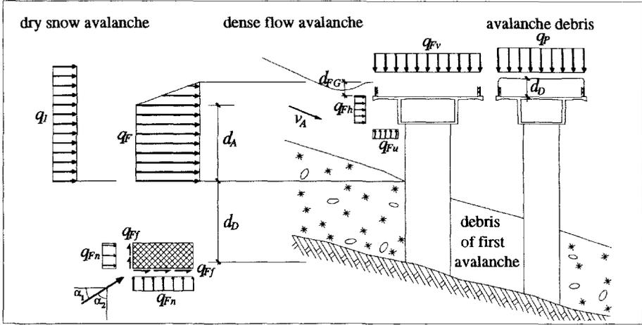
Fig. 4. Actions on piers and girders of the Reuss bridges A2 Wattingen, extreme hazard scenario
