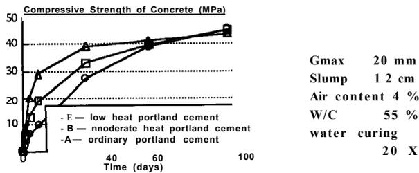
Fig 1 Strength of the Concrete using several kind of Cements
