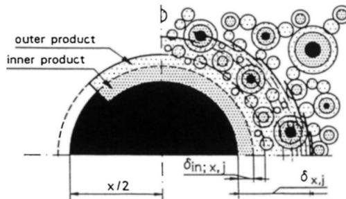
Fig. 2. Interaction mechanism for expanding particles. Left part: free expansion, formation of inner and outer product. Right part: embedding of particles, several stages.
