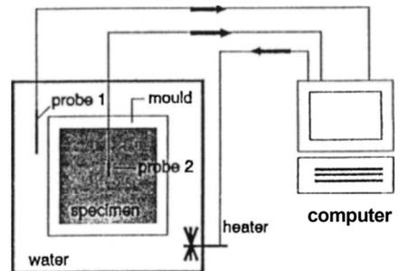
Fig. 3 Adiabatic test device Schematic.
