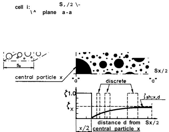
Fig. 1. Cell concept and shell density factor  $f_{sh;x,d}$
