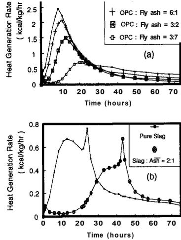
Fig.2 Effect of fly ash on conduction calorimetry.
