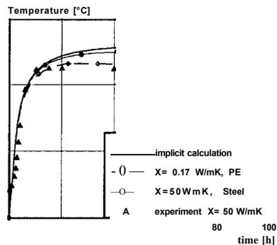
Fig. 5. Effect of type of mould on adiabatic hydration curves (explicit steering).
