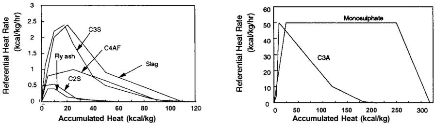
Fig.3 Assumed referential heat generation rate of cement clinkers and pozzolans.
