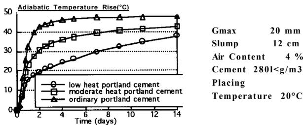
Fig. 2 Adiabatic Temperature Rise of the Concrete
