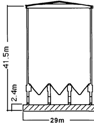
Fig. 3 Section of the Silo
