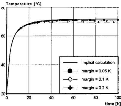
Fig. 4. Influence of steering accuracy of the adiabatic test device.
