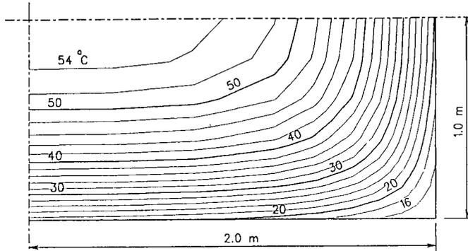
Fig.1. Temperature contour in a quadrant of a 2x4m column 72 hours after casting. (400kg/m<sup>3</sup> of ordinary cement, steel formwork).
