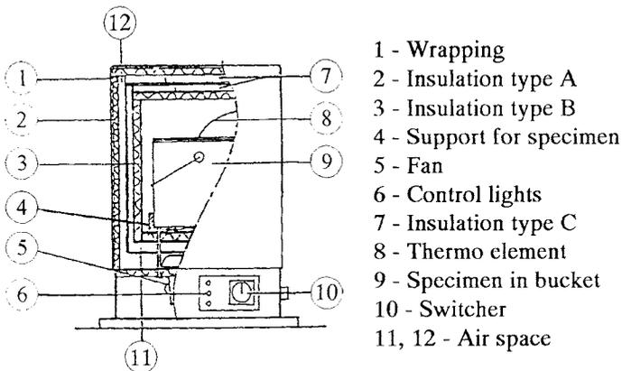
Fig. 1.7 Section of the Stema calorimeter.
