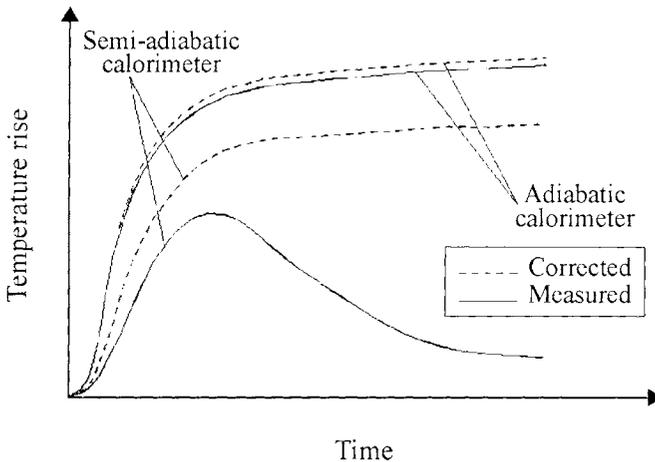
Fig. 1.9 Measured and corrected curves from adiabatic and semi-adiabatic tests.
