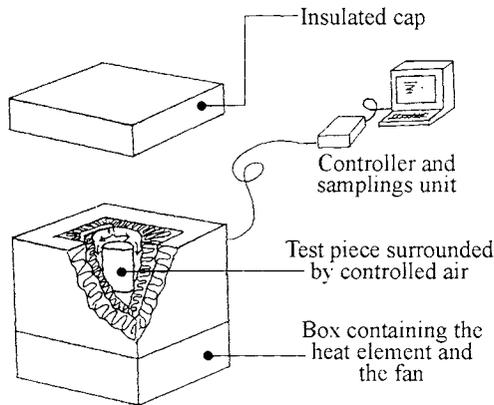
**Fig. 1.4** Adiabatic calorimeter developed in Luleå University.
