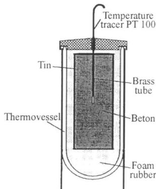
**Fig. 1.8** Semi-adiabatic calorimeter developed by Grube.
