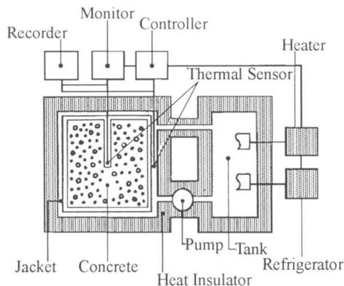
**Fig. 1.1** Adiabatic calorimeter of the Sumitomo Cement Company.
