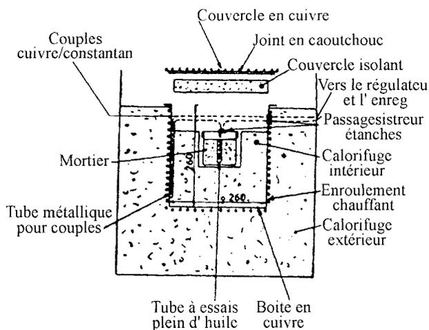
**Fig. 1.5** Sketch of the CERILH calorimeter
