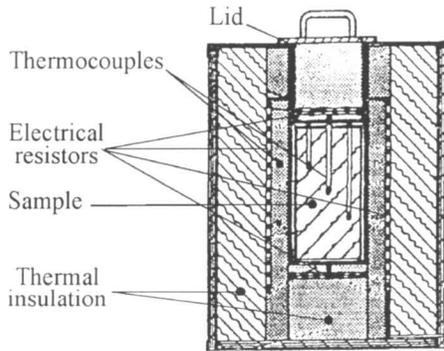
**Fig. 1.6** Adiabatic calorimeter developed by Costa.
