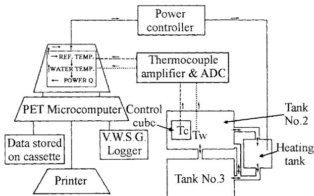
**Fig. 1.3** Control and logging system of the adiabatic calorimeter developed by Wainwright.
