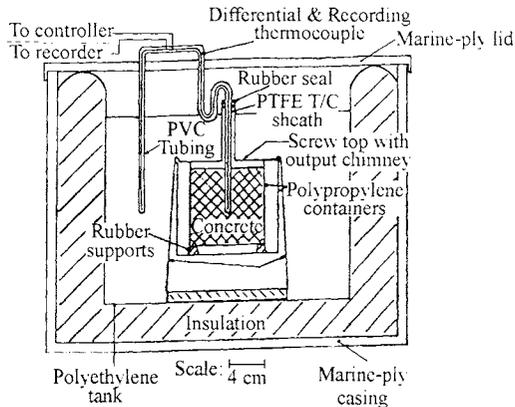
Fig. 1.2 Adiabatic calorimeter developed by Coole.
