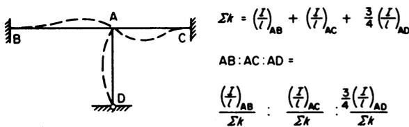
Figure 3.16 Distribution factors at typical joint
