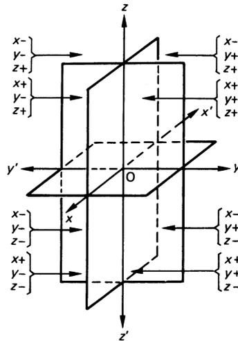
Figure 1.40 Sign conventions in analytical solid geometry
