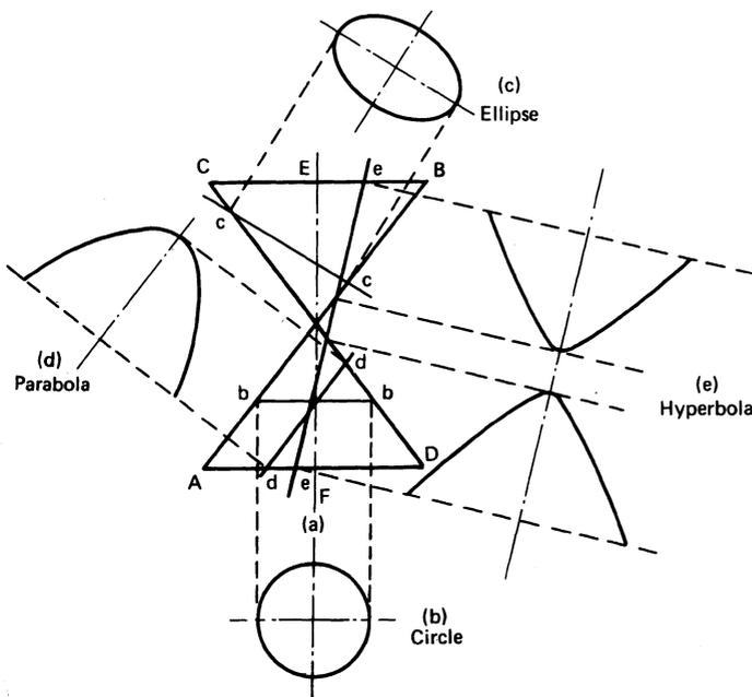
**Figure 1.35** Circular cones generated by two intersecting straight lines
