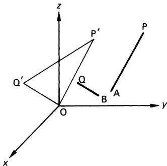
Figure 1.44 Angle between two lines of known direction-cosines
