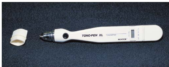
Figure 1.26 Tono-Pen with cover. The average IOP reading is displayed.
