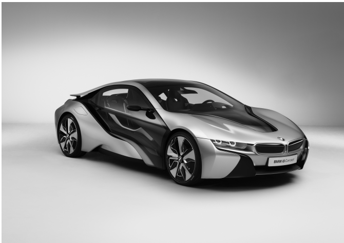
The i8 concept car, a hybrid sports car requiring three liters per 100 km and acceleration from 0 to 100 km/hr in under five seconds. Source: Courtesy of BMW.
