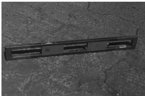
FIGURE 1.6 First commercial unit (circa 1980) of the Geonics EM-38 single dipole electromagnetic induction conductivity meter. (Courtesy of Dennis Corwin.)
