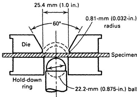
**Figure 21** Schematic of Olsen cup test. (From ASTM E290.)
