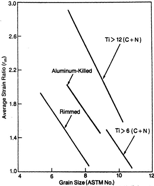
**Figure 18** A relationship between the  $r_m$  value and grain size of steel. The normal range of conventional rimmed and killed steels is shown. In addition to chemical composition, the value is determined by the coil processing. Two titanium-treated aluminum-killed steels are also shown. To produce an interstitial-free steel with a high  $r_m$  value, the amount of titanium present must exceed six times the amount of carbon plus nitrogen. (From Ref. 2.)
