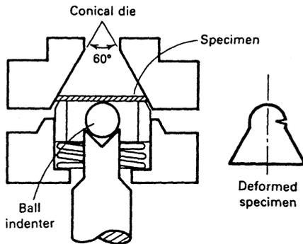
**Figure 25** Schematic of the Fukui conical cup test. (From Ref. 65.)
