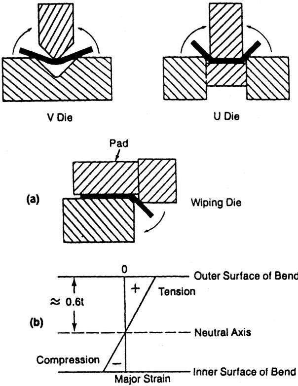
**Figure 1** Schematic diagrams showing (a) the action of a V-die, U-die, and a wiping die, and (b) the strain states in bending. (From Ref. 11.)
