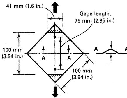
**Figure 29** Schematic of the Yoshida buckling test. (From Ref. 68.)
