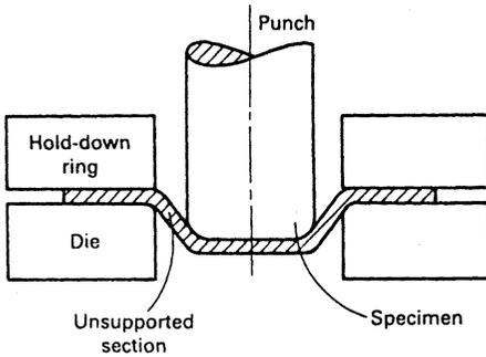
**Figure 26** Schematic of the conical cup wrinkling test. (From Ref. 1.)
