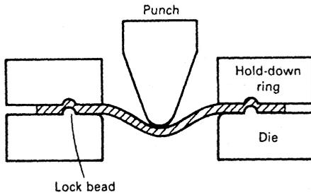
**Figure 20** Schematic of a stretch–bending test. (From Ref. 1.)
