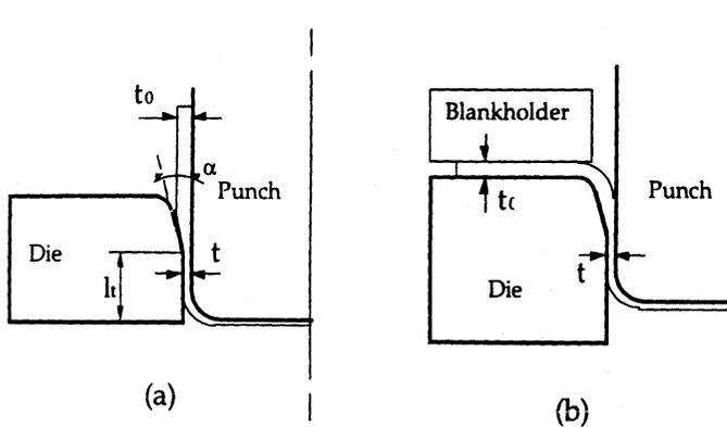
**Figure 9** (a) Simple and (b) simultaneous ironing. (From Ref. 18.)
