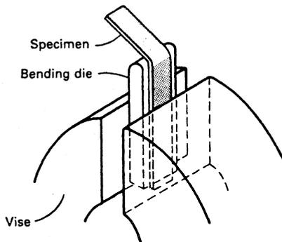
**Figure 19** Schematic of a simple bending test. (From ASTM E290.)
