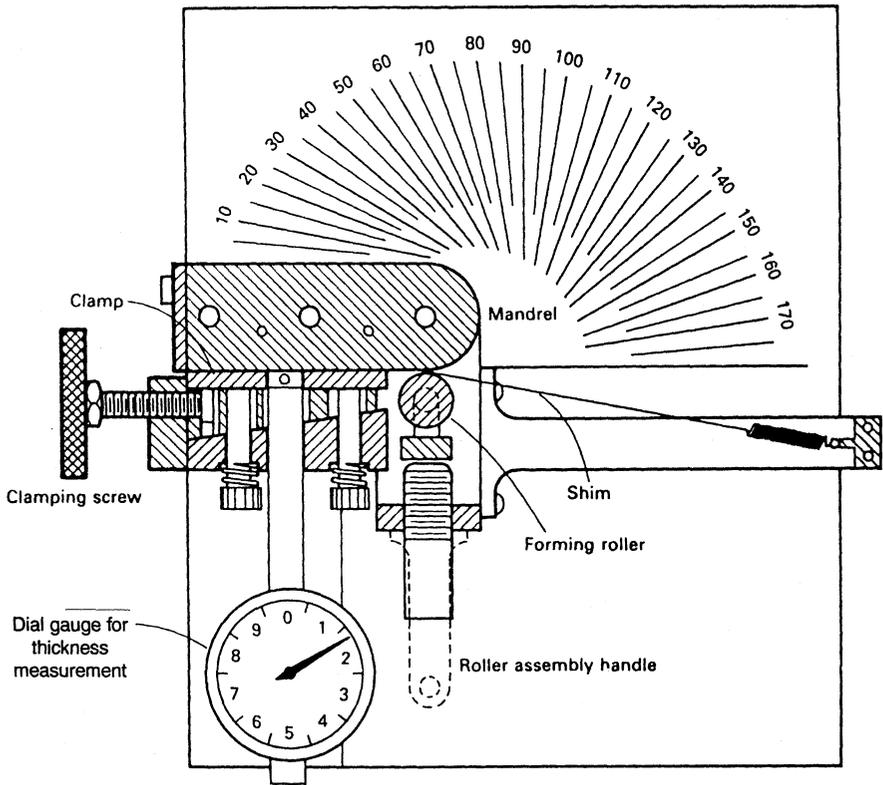
**Figure 30** Springback tester for determining yield strength. (From Ref. 74.)
