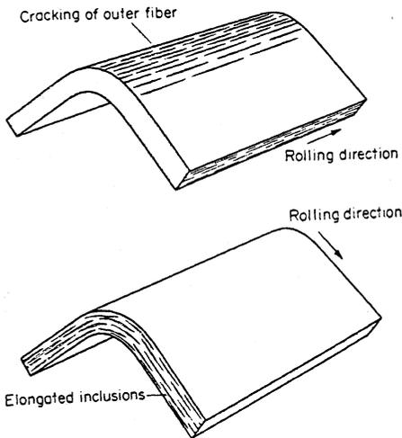
**Figure 13** Mechanical fibering in sheet metal and its effect on bending of sheet. (From Ref. 3.)
