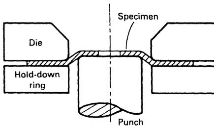
**Figure 23** Schematic of the hole-expansion test with a flat-bottomed punch. (From Ref. 1.)
