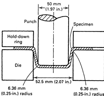
**Figure 24** Standard tooling for the Swift flat-bottomed cup test. (From Ref. 1.)
