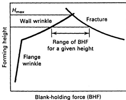
**Figure 27** Wrinkling and fracture limits in conical cup drawing test. (From Ref. 68.)
