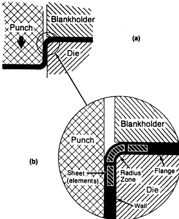
**Figure 4** Schematic diagram showing bend-and-straighten operation. (From Ref. 2.)
