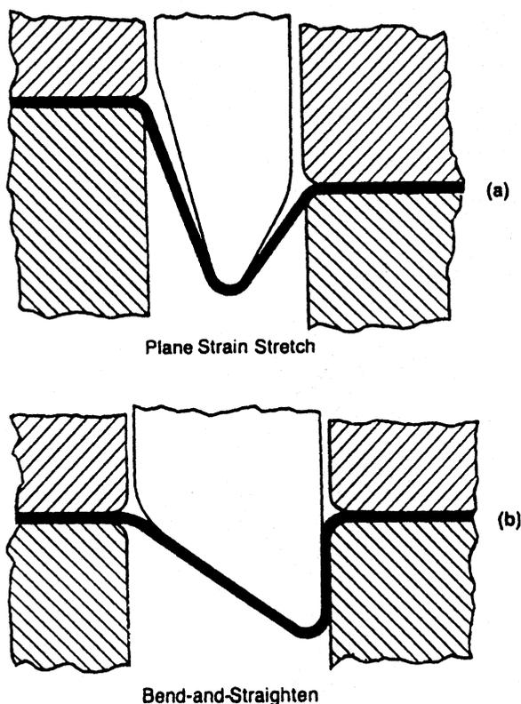
**Figure 6** The die angle can change the deformation mode from (a) plane-strain stretch to (b) bend-and-straighten. (From Ref. 2.)
