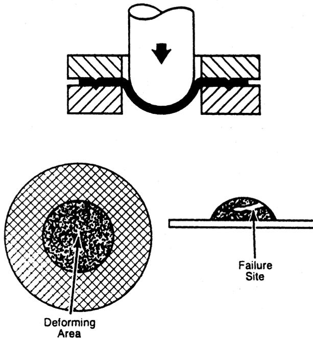
**Figure 5** Stretch forming in which no deformation is allowed in the flange area and all deformation occurs in the die opening over the punch. (From Ref. 2.)
