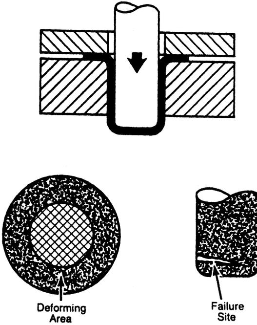
**Figure 7** Deep drawing in which no deformation occurs over the bottom of the punch and all deformation is restricted to a tension-compression deformation in the flange of the blank. (From Ref. 2.)
