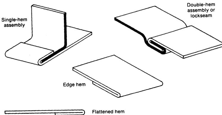
**Figure 2** Assembly of sheet metal panels by hems and seams. (From Ref. 13.)
