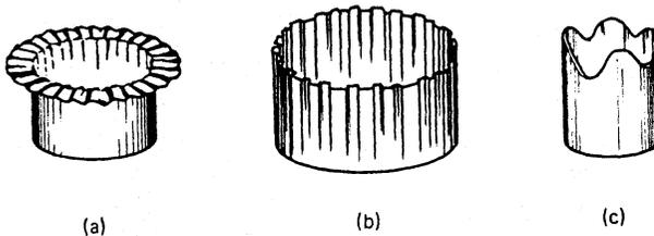
**Figure 10** Defects occurring in deep-drawing operations: (a) wrinkling in the flange, (b) wrinkling in the wall, and (c) earing. (From Ref. 20.)
