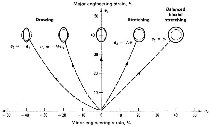
**Figure 8** Schematic diagram of several major strain/minor strain combinations. (From Ref. 1.)
