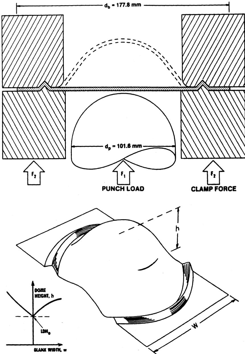
**Figure 22** Dome test and limiting dome height test. Punch diameter: 101.6 mm; punch rate: 4.2 mm/s; clamp force: 1000 kN, no. of replicates: 5. (From Refs. 57 and 61.)
