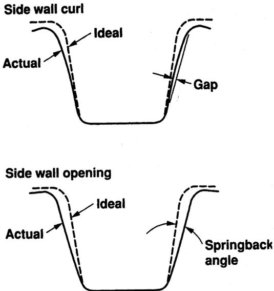
**Figure 11** Modes of springback in plane-strain channel forming. (From Ref. 25.)
