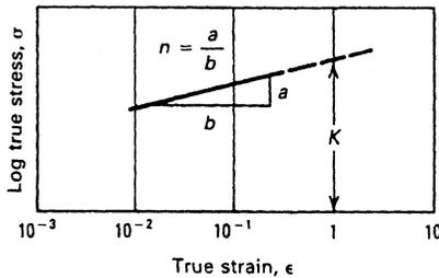
**Figure 17** A log  $\sigma$  versus log  $\epsilon$  plot for the true stress–true strain curve. (From Ref. 28.)
