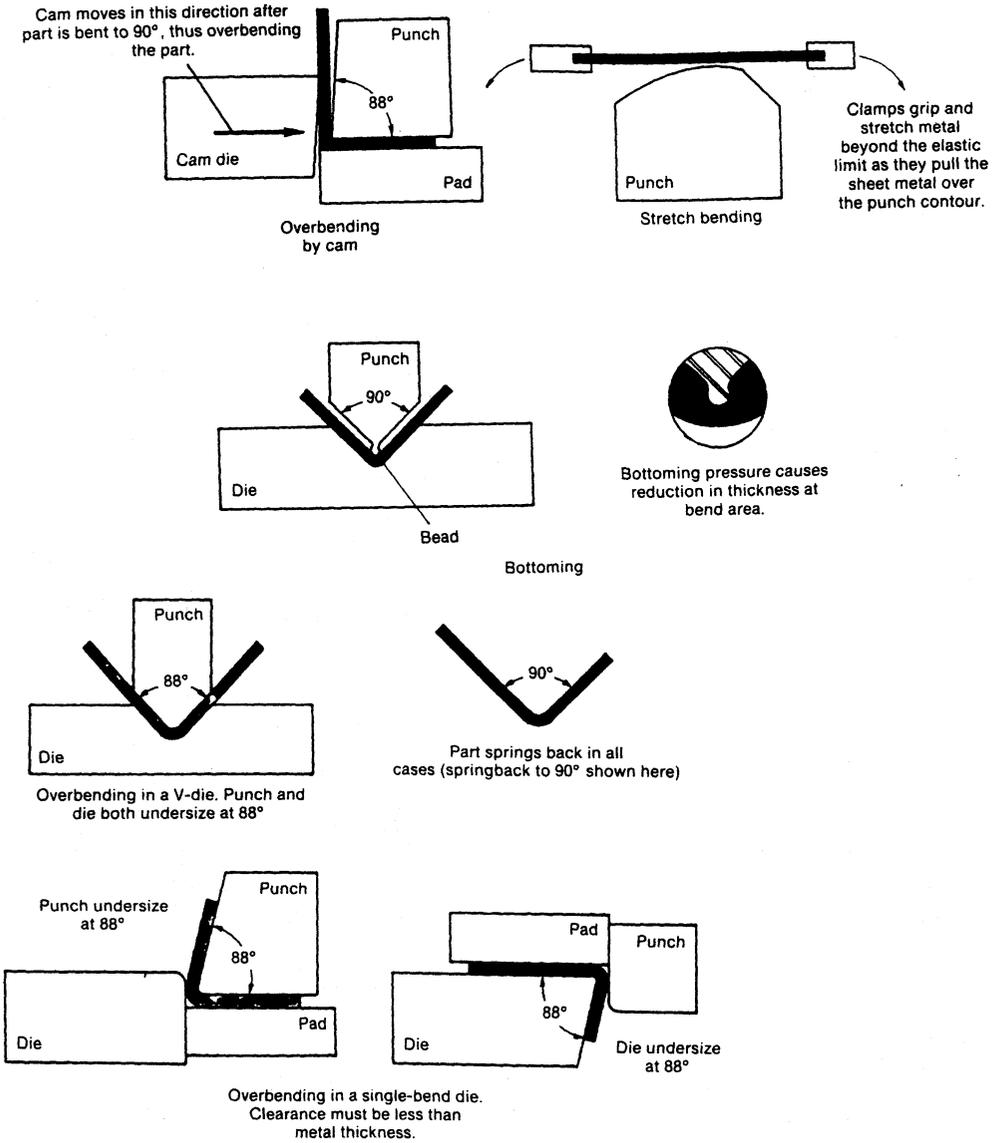
Figure 12 Methods of overcoming springback. (From Ref. 11.)
