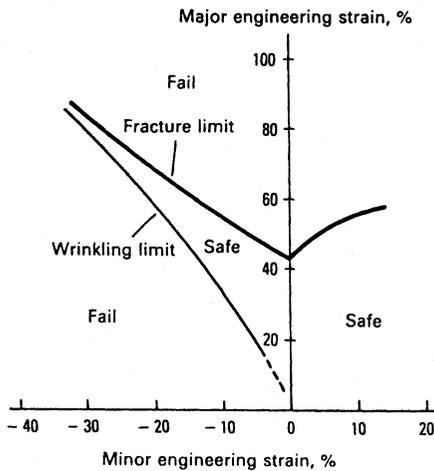
**Figure 28** Combined forming and wrinkling limit diagram. (From Ref. 69.)
