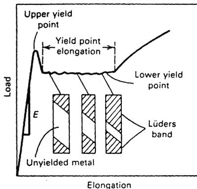
**Figure 15** Schematic showing yield-point elongation. (From Ref. 32.)
