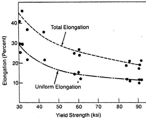
**Figure 16** Effect of yield strength on both uniform elongation and total elongation. (From Ref. 2.)
