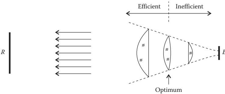
**FIGURE 1.21** Collimator optics with emitter  $E$  and receiver  $R$ . Optimum optic at the center. To the left, optics are efficient, but large. To the right, optics are small but inefficient.
