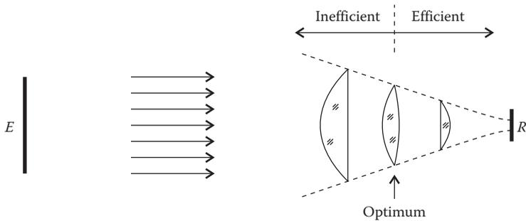
**FIGURE 1.22** Concentrator optics with emitter  $E$  and receiver  $R$ . Optimum optic at the center. To the left, optics are large but inefficient. To the right, optics are efficient but small.
