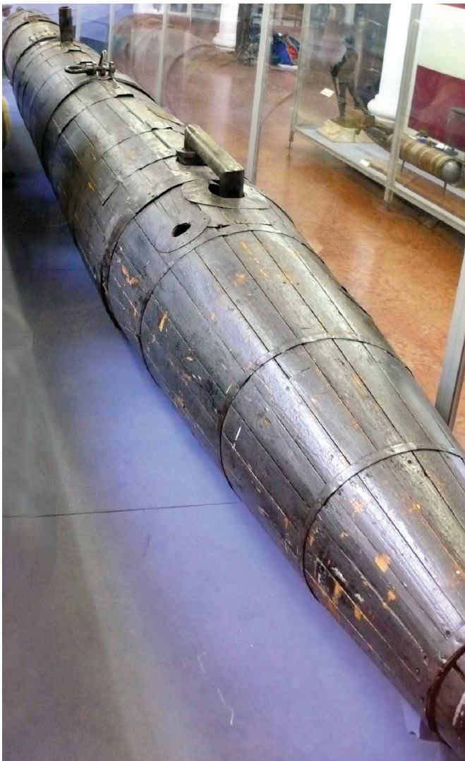
The tail of the Mignatta, showing the wooden construction held together with brass hoops.
