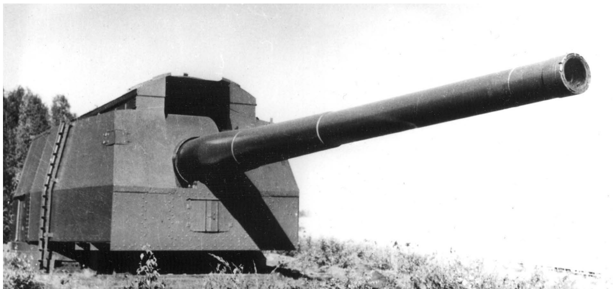
The 406mm gun on a test mounting at the proving grounds near Leningrad. Trials of the first gun were carried out 6 July to 2 October 1940 and were deemed successful. The trials gun was subsequently replaced by another, and from 29 August 1941 this gun was used to bombard German positions during the siege of Leningrad. A total of twelve barrels were manufactured by the Barrikada Works in Stalingrad. (Boris Lemachko collection)
