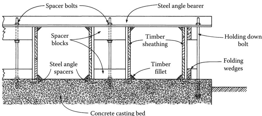
Figure 2.8 Timber formwork for precast concrete piles.
