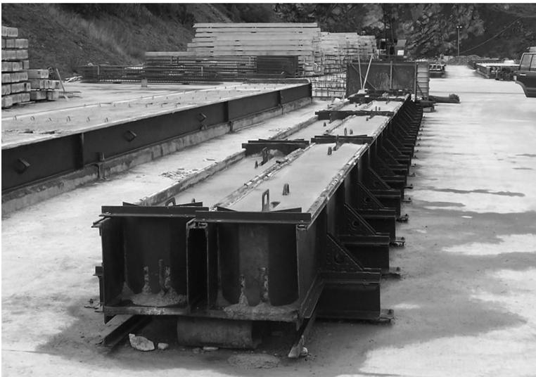
Figure 2.10 Steel moulds in pile casting yard.
