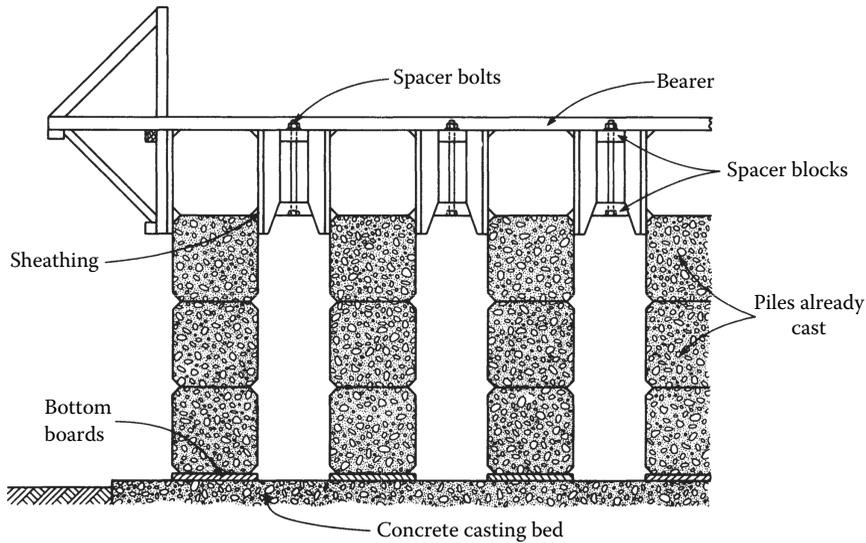
Figure 2.9 Casting precast concrete piles in tiers.
