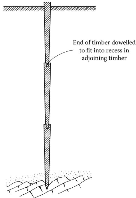
Figure 2.4 Splicing timber piles in multiple lengths.
