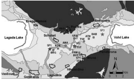
Figure 10. Map with the surface accelerographs (green rectangles) and the geological background ( http://euroseis.civil.auth.gr , Pitilakis et al. 1999).
