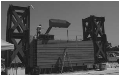
Figure 5. UCSD NEES large high performance outdoor shake table (LHPOST), with soil container on shake table during model construction.
