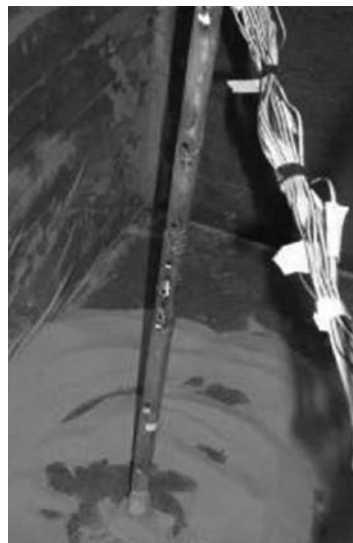
Figure 4. Strain gauged pile.
