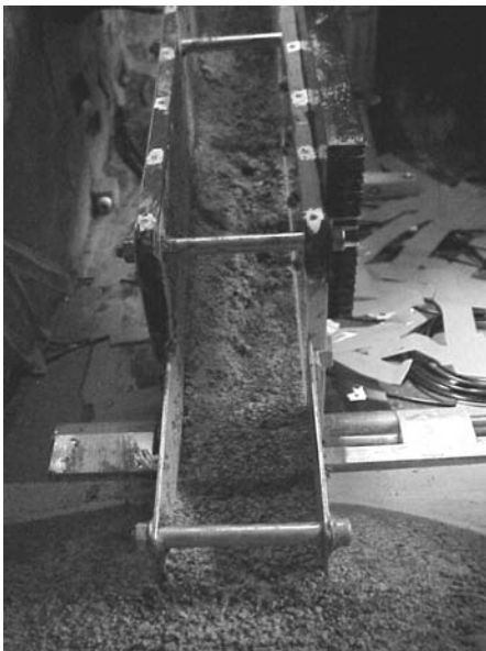
Figure 5. Aftermath of erodible bed debris flow experiment on the ETH Zurich drum centrifuge carried out at a centrifugal acceleration equivalent to 40 g (approx.). Photo is taken from the bottom fan area of the horizontally mounted flume. Earth's gravity acts in the leftward direction relative to the picture.
