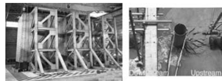
Figure 24. The NIED large size laminar box (Kagawa et al. 2004), and passive bulge of soil upslope of the flexible pile due to liquefaction-induced lateral ground displacement (He 2005).
