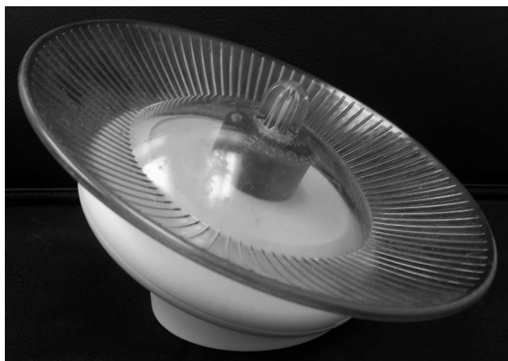
FIGURE 2.30 Low-profile wheel. Flat running wheels (or discs) must replace standard running wheels when research is conducted on tethered rodents. (Photo by R. Refinetti.)
