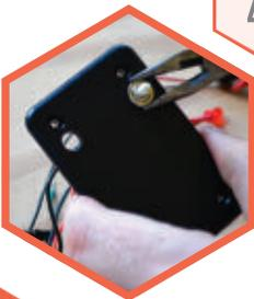
Drill a 5/16" hole in the top right of the enclosure lid, just below the lid's screw hole. Drill a 1/4" hole in the top left, also below the lid's screw hole. Insert the LED holder into the 1/4" hole from the outside and the LED into the holder from the inside. Remove the plastic button, mount the switch body into the 5/16" hole with its bundled hardware, tighten down and reattach the button.
