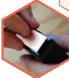
Cut a 3/4" x 1-1/2" strip of copper-clad board with a rotary tool and stick it to one end of the enclosure with double-sided tape. Drill a 1/16" hole through both copper and case near the middle of the strip. Thread the green wire from the perfboard through the hole from inside, bend it over and solder it to the copper.
