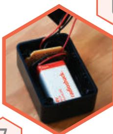
Clip a battery to the connector and insert it, along with the perfboard, into the enclosure body. Orient the solder side of the perfboard toward the battery. Route any excess wire and gently close the lid. Screw it in place.
