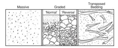
FIG 2.1 Massive and graded bedding (after Fritz and Moore 1988).
