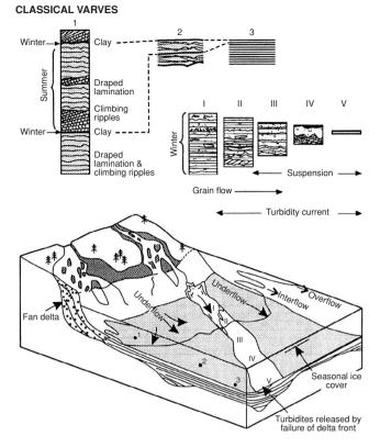
FIG 2.2 Rhythmite deposition in lake environments (modified from Eyles and Miall 1984).
