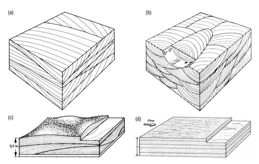
FIG 2.3 Sand and gravel cross-bedding with reactivation surfaces marked in bold: a) planar cross-bedding; b) trough crossbedding; c) hummocky cross-stratification (HCS); d) plane beds (after Harms *et al.* 1982).
