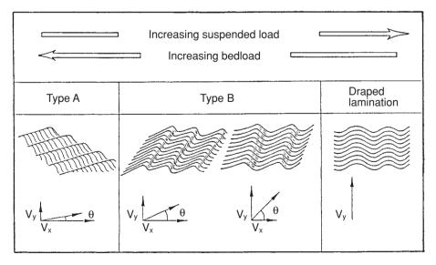
FIG 2.4 The production of ripple cross-lamination. Ripples climb at angle  $\Theta$  whose tangent is the mean aggradation rate V<sub>y</sub> divided by the downstream migration rate V<sub>y</sub> (from Ashley *et al.* 1982).
