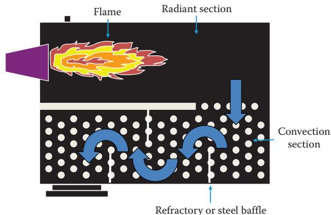
**FIGURE 1.1** Flow through a boiler, highlighting radiant and convection sections.
