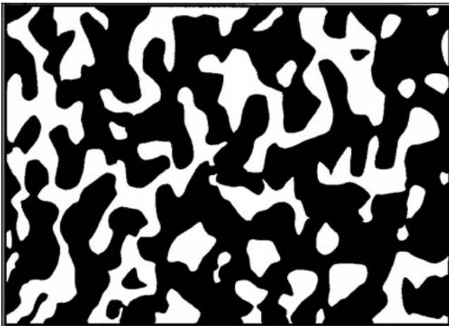
**FIGURE 1.6** Skeletal microstructure of FGM material. (From Vel, S.S. and Batra, R.C., *AIAA J.*, 40, 1421, 2002. With permission.)
