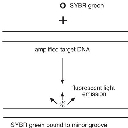
**Figure 1.7** Mechanism of SYBR green fluorescence. SYBR green dye binds to the minor groove of the DNA double helix. The unbound dye emits little fluorescence, which is greatly enhanced when bound to DNA.
