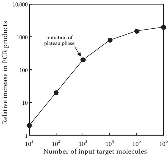
**Figure 1.2** Dependence of PCR product accumulation on number of input targets from 35 amplification cycles.
