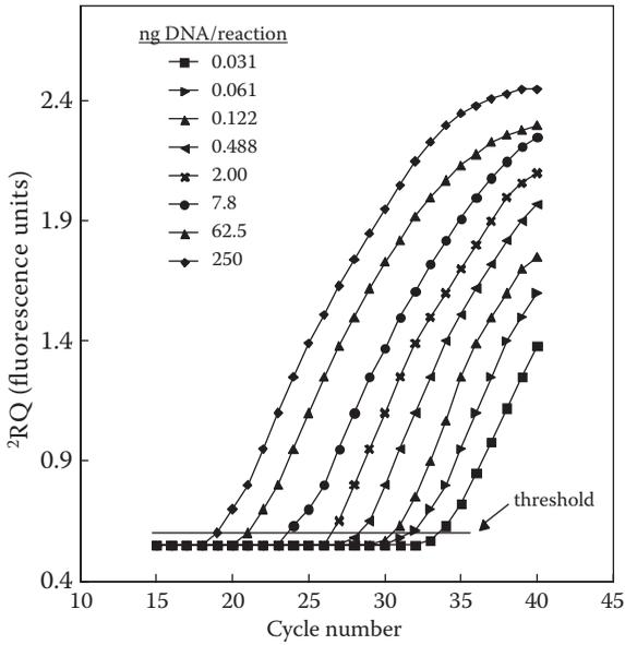
**Figure 1.13** Appearance of real-time PCR screen display of thermal cycling plots of target DNA amplification. Decreasing the quantity of target DNA results in an increased number of cycles required to detect fluorescence above the threshold level (shift of the plot to the right).
