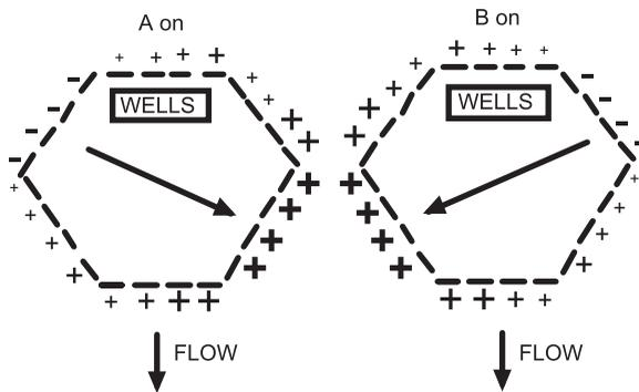
**Figure 1.16** Voltage clamping by the CHEF-DR-II system. A: Relative electrode potentials when the +60 volt field vector is activated. B: Relative electrode potentials when the -60 volt field vector is activated.
