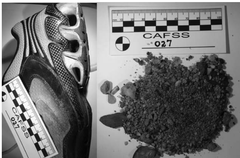
Figure 1.2 Contact traces of yellowish-gray soil on the suspect's shoes (left) and the control soil specimen from the bank of a river (right), which comprises a mixture of 95% coarse gravel and rock fragments and only 5% clay and silt ( < 50 \mu\text{m} fraction). (See color insert following p. 178.)
