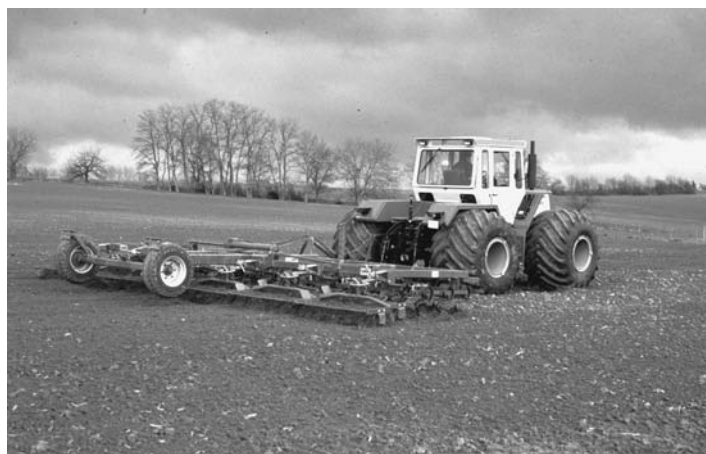
Figure 1.6 For seedbed preparation on lighter soils, one pass with a drawn harrow is sufficient.
