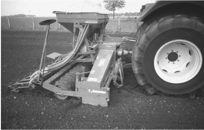
Figure 1.7 In western Europe, PTO-driven harrows are very popular for seedbed preparation after plowing on heavy soils.
