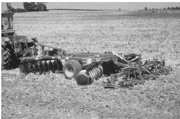
Figure 1.2 Disk harrows provide a good mixing of soil and straw.
