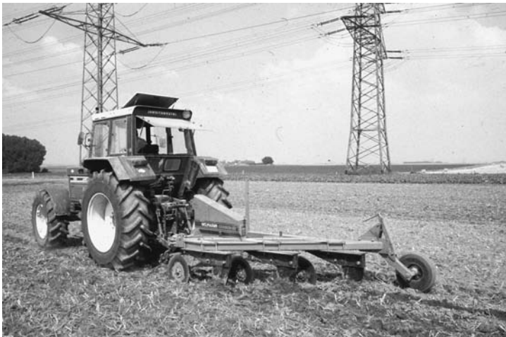
Figure 1.5 Special implements like the “paraplow” provide sufficient soil loosening without turning and mixing.
