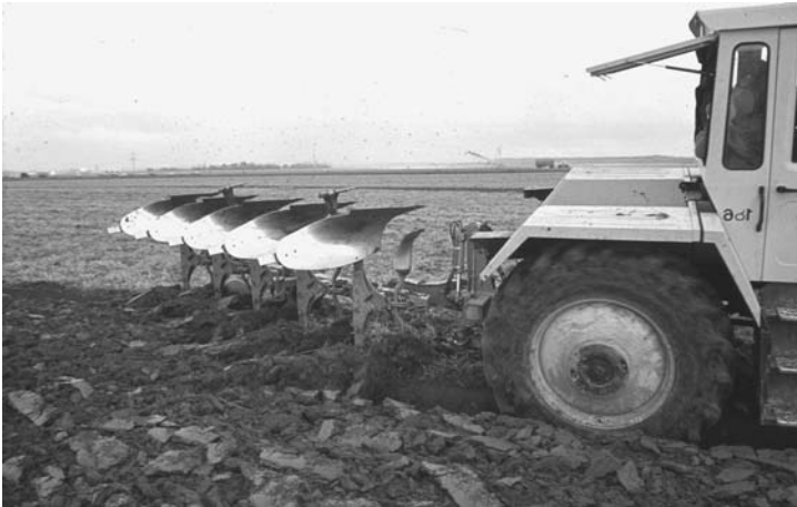
Figure 1.3 The use of mounted reversible plows is widespread in western Europe.
