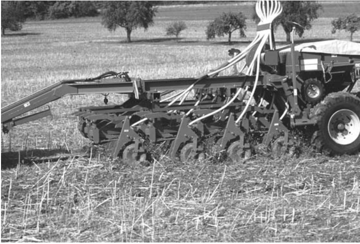
Figure 1.9 Hoe drills do a good job of direct seeding if the machine has adequate residue clearance.
