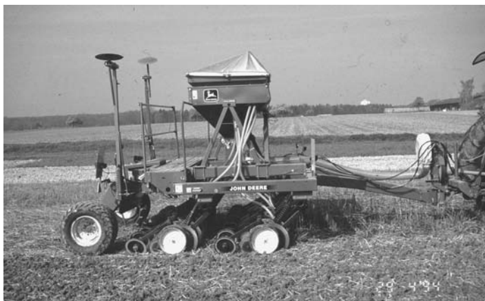
Figure 1.8 Single-disk drills require good residue management for maximum seedling emergence.
