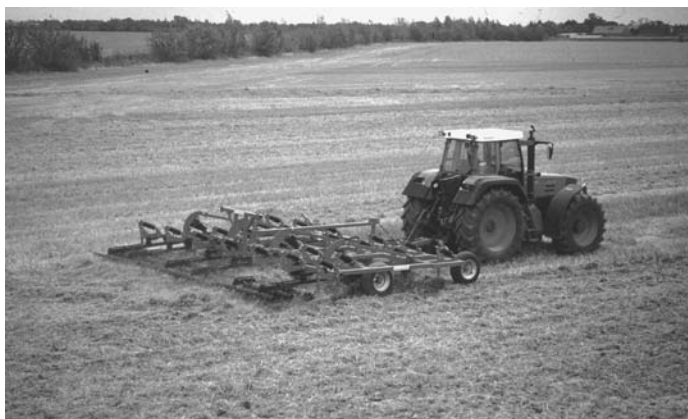
Figure 1.1 Cultivators fitted with additional disk runners have gained increasing importance.
