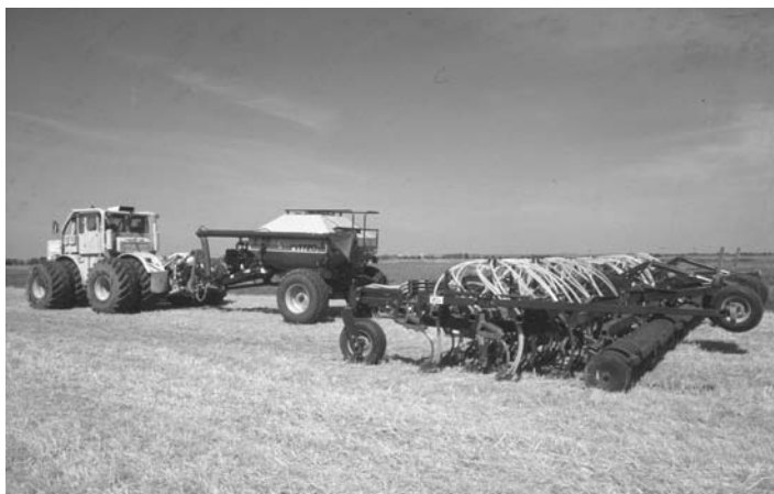
Figure 1.10 Air seeders have gained acceptance in areas where grain is cropped in large areas of land.
