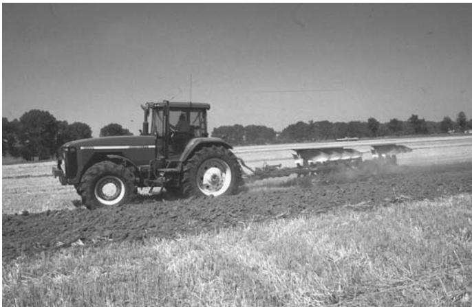
Figure 1.4 Semimounted reversible plows are growing in importance.
