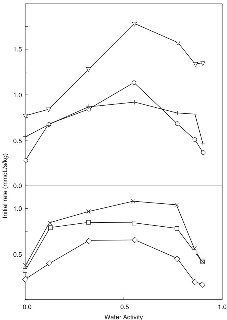
FIGURE 3.5 Activity of Lipozyme catalyst as a function of water activity in a range of solvents.<sup>24</sup> Hexane(▽), toluene(×), trichloroethylene(O), isopropyl ether(□), pentan-3-one(◇), and none, i.e., liquid reactant mixture(+).
