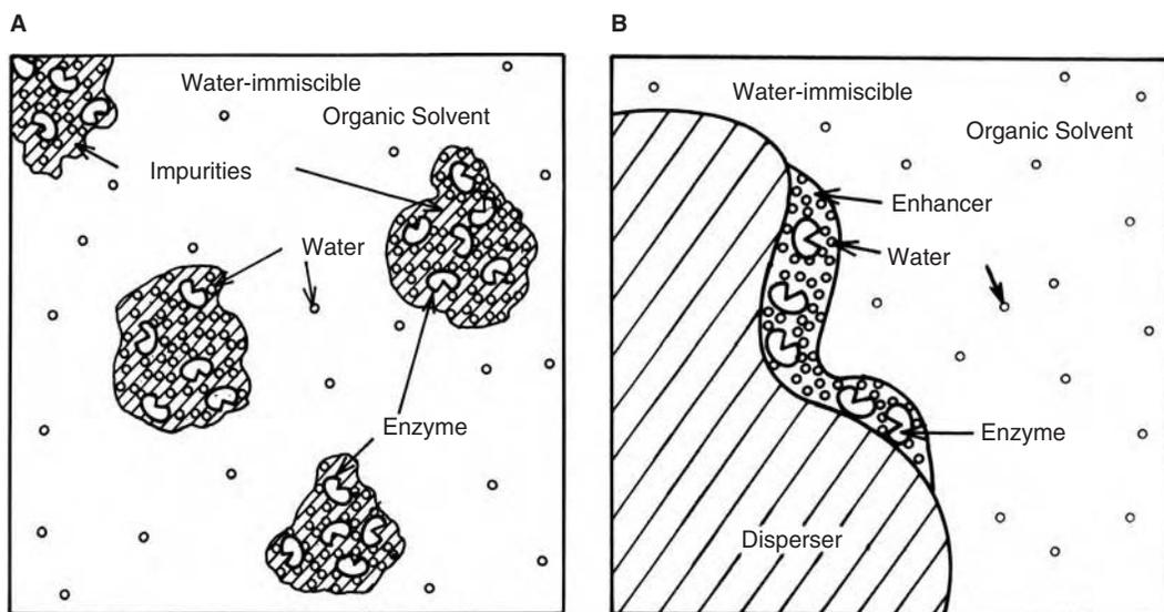
**FIGURE 3.1** Schematic pictures of crude enzyme powder particles suspended in microaqueous medium (a), and the system of (pure enzyme + activity enhancer) deposited on a disperser particle which is suspended in microaqueous medium (b).<sup>6</sup>
