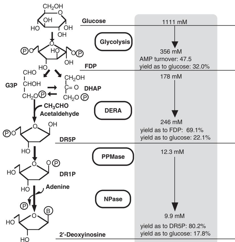
FIGURE 2.10 Biochemical retrosynthesis of 2'-deoxyribonucleoside.
