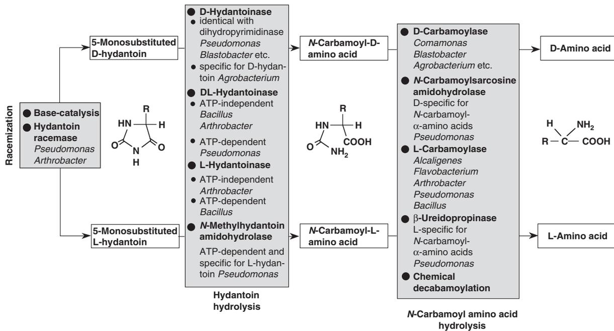
FIGURE 2.3 Processes for optically active  $\alpha$ -amino acid production with combinations of various hydantoin–metabolizing enzymes.
