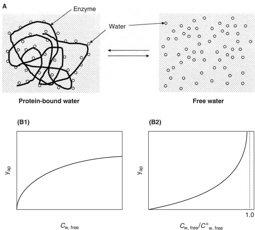
**FIGURE 3.4** Dynamic equilibrium between enzyme-bound water and free water in an organic medium (A), and general profiles of the adsorption isotherms of water between the enzyme and water-miscible organic solvent (B1) and between enzyme and water-immiscible organic solvent (B2).<sup>20</sup>  $C_{w, free}^*$  is water solubility of the organic solvent.
