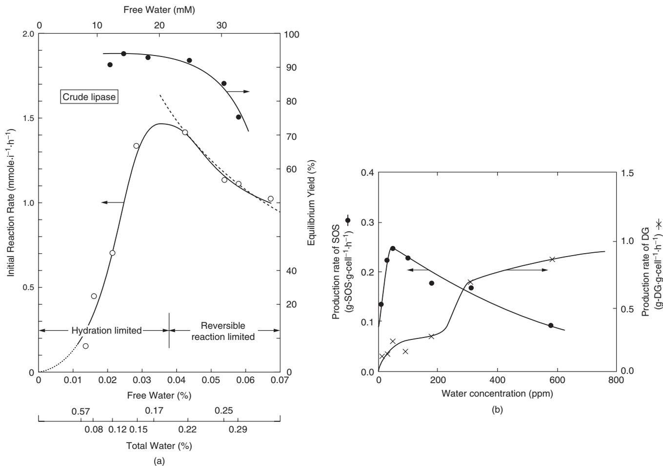
FIGURE 3.3 Effect of trace amount of water on lipase-catalyzed esterification (a)<sup>13</sup> and transesterification (b).<sup>30</sup>
