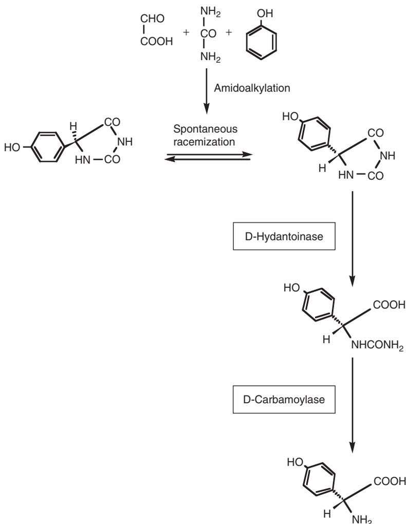
FIGURE 2.4 Industrial process for D-p-hydroxyphenylglycine production with hydantoin-metabolizing enzymes.
