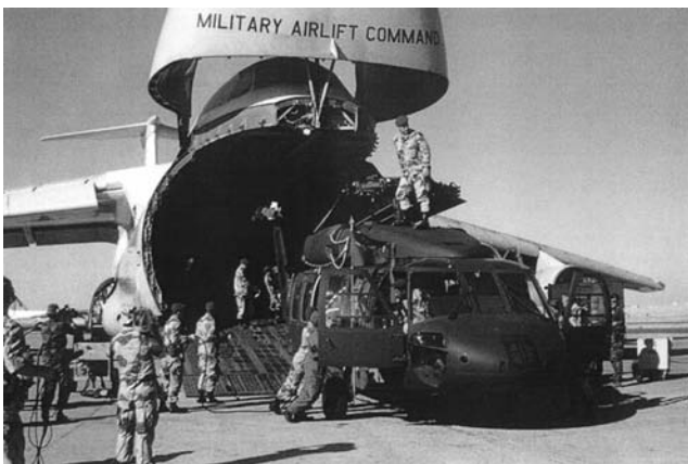
Figure 12 C-5 Galaxy. The largest cargo aircraft in the U.S. inventory, it can carry a payload of 260,000 lb and has a fully loaded range of 2160 nautical miles. It is refuelable in the air. Original model became operational in 1970. The C-5 is being upgraded to continue service to a projected date of 2040. Source: Courtesy of Ref. 57.
