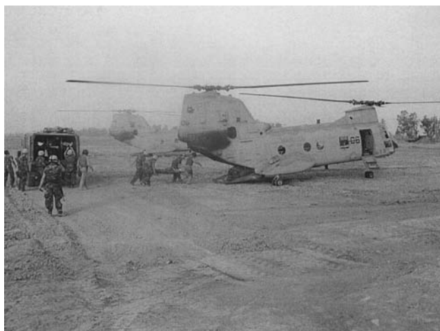
Figure 9 CH-46 USMC helicopter. This image shows the U.S. Marines loading casualties onto the CH-46 on an unimproved airfield outside Ramadi, Iraq. The CH-46 is an all-weather, day/night, night vision goggle helicopter used by marines for MEDEVAC, assault, transport of combat troops, supplies, and equipment during amphibious and subsequent operations ashore. As a medical evacuation platform it is capable of holding 15 litters and two medical attendants in addition to the normal crew of four to five (normal crew: four—pilot, co-pilot, crew chief, and 1st mechanic; combat crew: five—pilot, co-pilot, crew chief, and two aerial gunners). Used in theatre for transport of casualties medium-range [i.e., level II medical treatment facilities to Level III or to ship (which may have level III equivalent)]. Source: Courtesy of Joseph F. Rappold, CDR, U.S. Navy.
