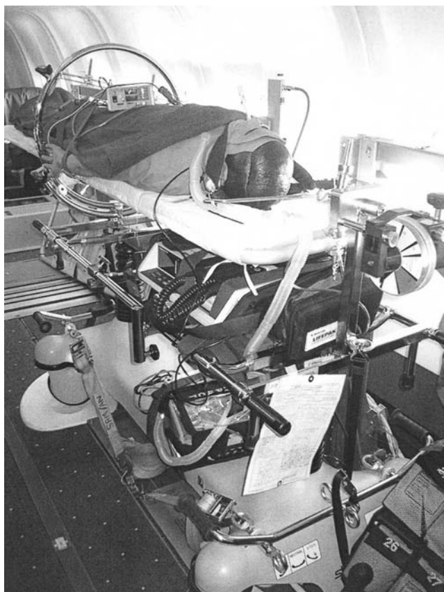
Figure 7 A standard spinal immobilization bed has been reconfigured for use inside an aircraft. This device allows a secure immobilization, inline stabilization, and the ability to rotate the patient to prone position while in flight. Source: Courtesy of Maureen McCunn, Maryland, U.S.A.
