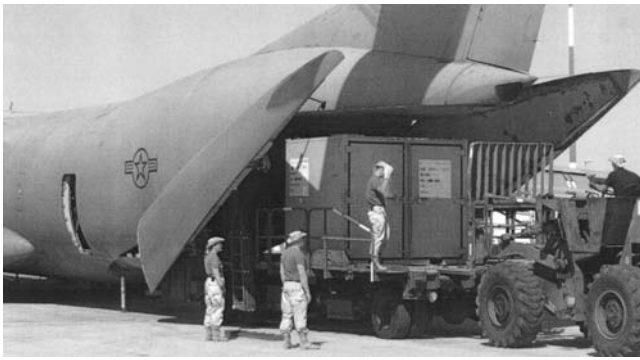
Figure 11 C-141 Starlifter. The C-141 was the first jet-powered cargo aircraft for the U.S. Air Force, starting in 1964. It has gradually been getting retired and is currently only operational in two Air National Guard units. It was the first intercontinental jet cargo aircraft that could be refueled in midair. Maximum payload is 94,500 lb, and maximum payload range is 2175 nautical miles. Source: Courtesy of Ref. 56.
