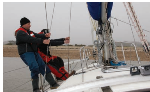
On the 40ft Crash Test Boat, three 'heavies' on the shrouds didn't induce much heel
