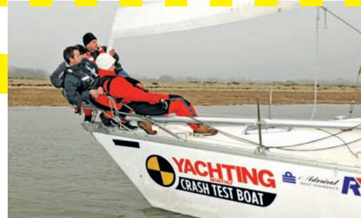
Weight forward reduces draught on bilge and long keelers
