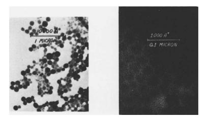
(I, II) Electron micrographs of alkyd-in-water microemulsions: (I) average diameter of droplets 1200Å. Magnification 17,000 X taken at 10,000 X; (II) average diameter of droplets 300Å. Magnification 140,000 X taken at 80,000 X. (III) Phase equilibria diagram representing four component micellar solutions of Friberg school. (I and II reproduced from Prince, L. M., "Carnauba Wax Molecules," Soap and Chemical Specialities, September, October, 1960, courtesy MacNair, Dorland, Inc.)
