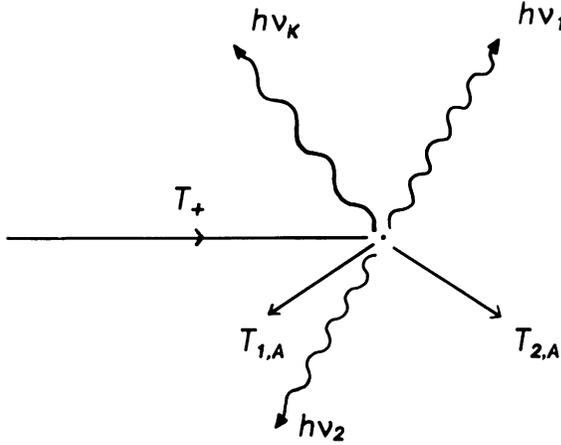
**Fig. 3.** A positron with kinetic energy  $T_+$  annihilates with an atomic electron giving rise to two annihilation photons with energies  $h\nu_1$  and  $h\nu_2$ . In subsequent deexcitations of the electronic structure, a characteristic roentgen ray with energy  $h\nu_k$  and two Auger electrons with kinetic energies  $T_{1,A}$  and  $T_{2,A}$  are emitted.
