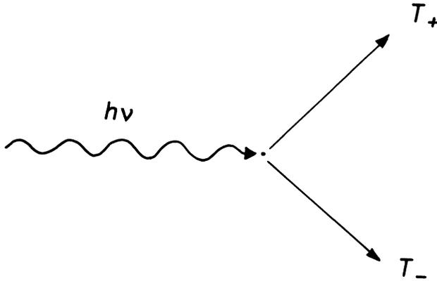
Fig. 2. A photon of energy  $h\nu$  is absorbed in the field of an atomic nucleus by emission of a positron and a negatron (pair production) with kinetic energy  $T_+$  and  $T_-$ . [After Alm Carlsson (1979).]
