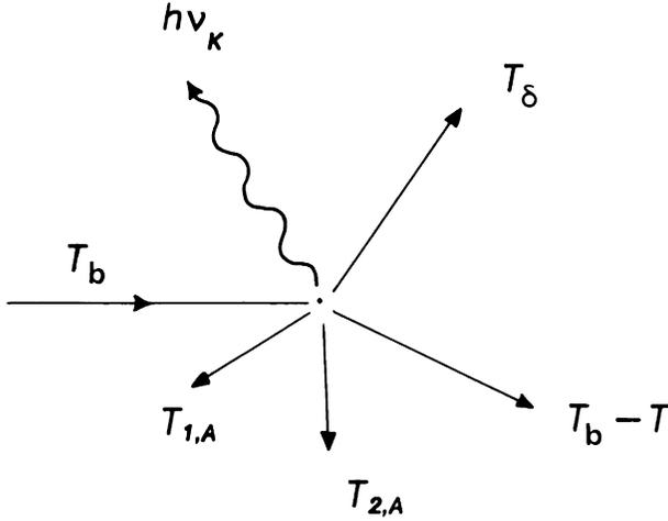
**Fig. 1.** A charged ionizing particle with kinetic energy  $T_b$  collides with an atomic electron and loses kinetic energy  $T$ . The atomic electron is knocked out and escapes with kinetic energy  $T_\delta$  ( $\delta$  particle). In the subsequent deexcitation of the electronic structure, one fluorescence photon with energy  $h\nu_k$  and two Auger electrons with kinetic energies  $T_{1,A}$  and  $T_{2,A}$  are emitted. [After Alm Carlsson (1979).]
